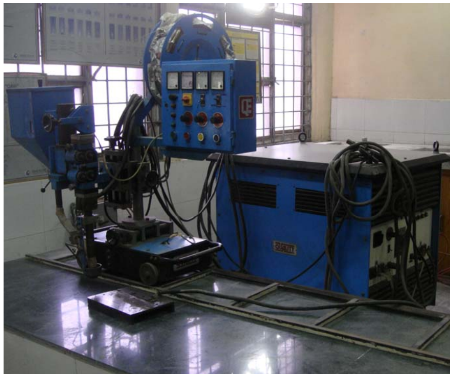
Fig 3.14 Picture of SAW machine used for experimental work courtesy Quality Engineers.
