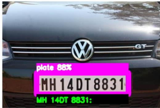
Fig 6.2. Optical Character Recognition of License Plates after OCR Model Implemented.
