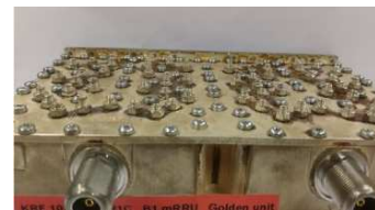
Fig. 1. A commercial MW filter
