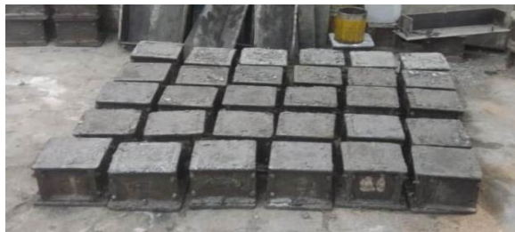
Figure 1 Casted cube specimens
