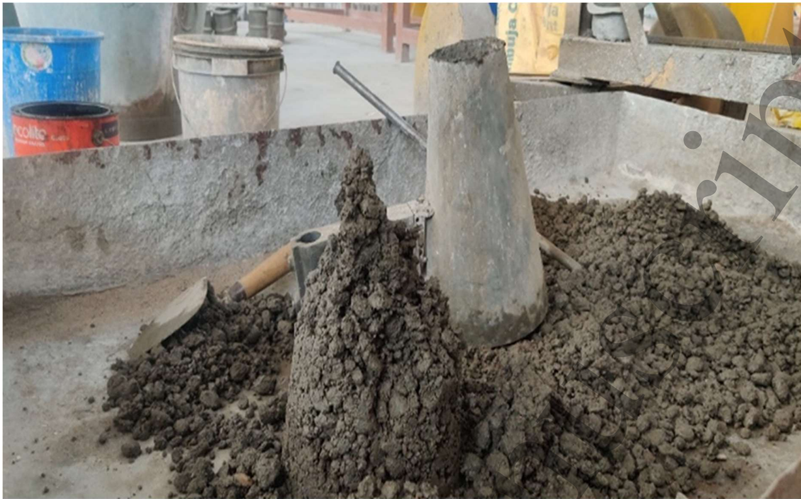
Figure 3 Picture during the slump test
