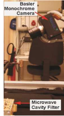
Fig. 10. Basler monochrome camera mounted with optical bandpass filters
