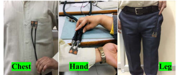
Fig. 17 On body scenario to measure S -parameters of the fabricated MIMO antenna prototype.
