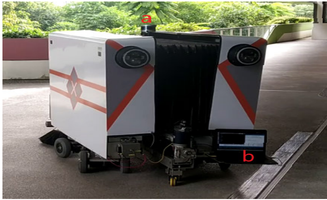
Fig. 12. PANTHERA experimental setup: a) LiDAR placement and b) workstation.
