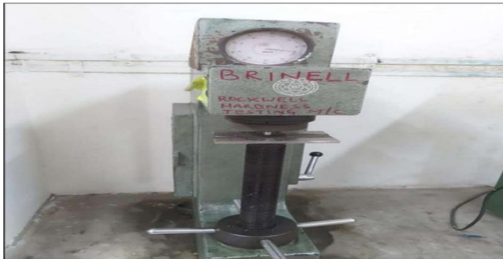
Figure 3 Measurement of the hardness using the Rockwell hardness testing machine
