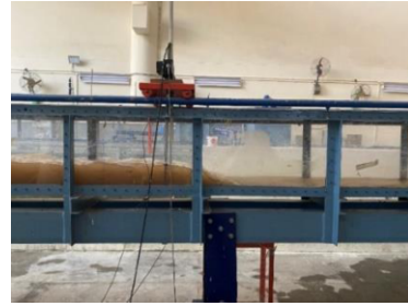
Figure 7. Occurrence of hydraulic jump in the rectangular flume.
