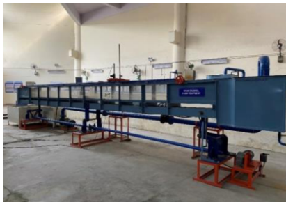
Figure 1. Rectangular flume used in this project placed in the Laboratory.
