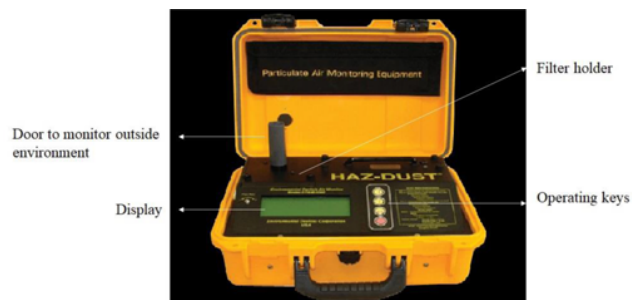
Figure 2. HAZ DUST EPAM 5000 Instrument used for RSPM test.
