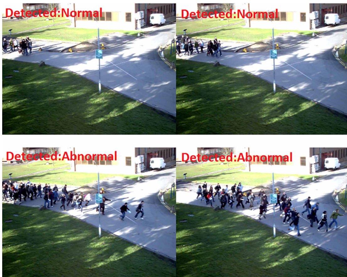
Figure 10. Detection results on PETS2009 (Time 14- 17)
