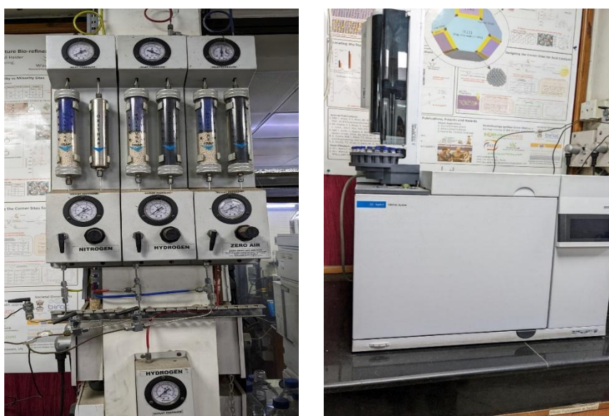
Figure 3.7. Gas chromatography for sample characterization
