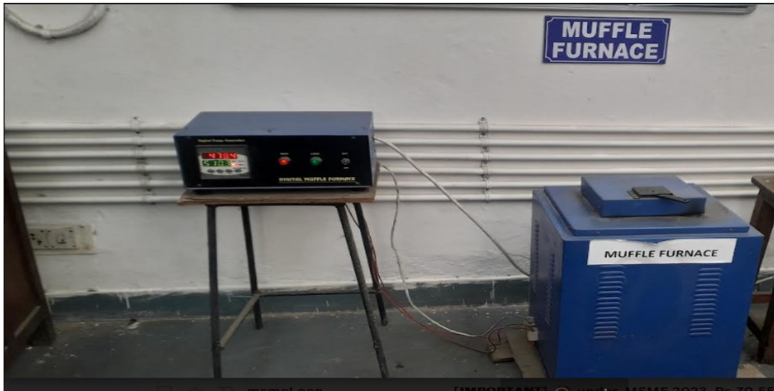
Fig.6: Tempering of EN-36C alloy steel in Muffle Electric furnace
