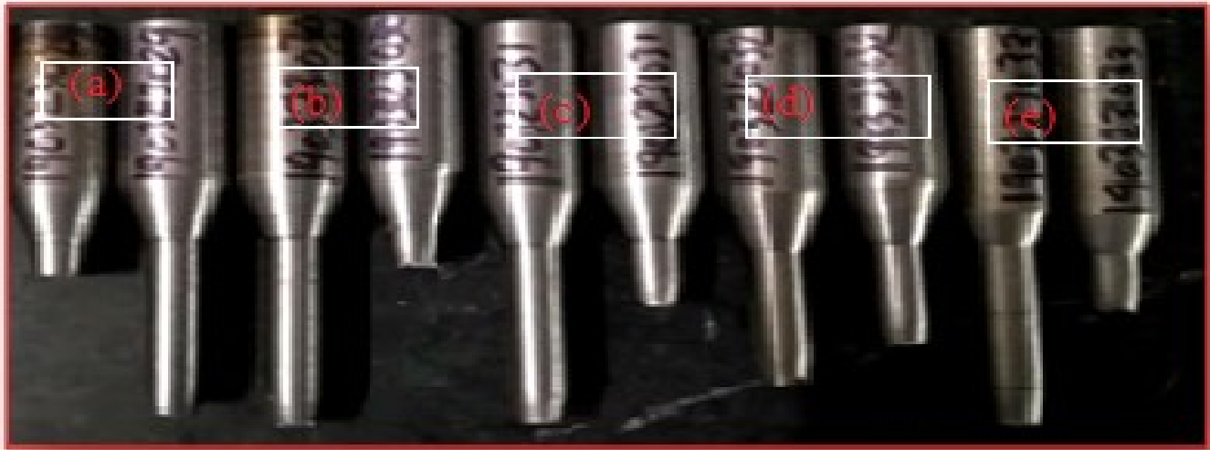
Fig.10: Broken test specimens (a) Untempered (b)Tempered at 200°C (c)Tempered at 300°C (d) Tempered at 500°C (e) Tempered at 700°C
