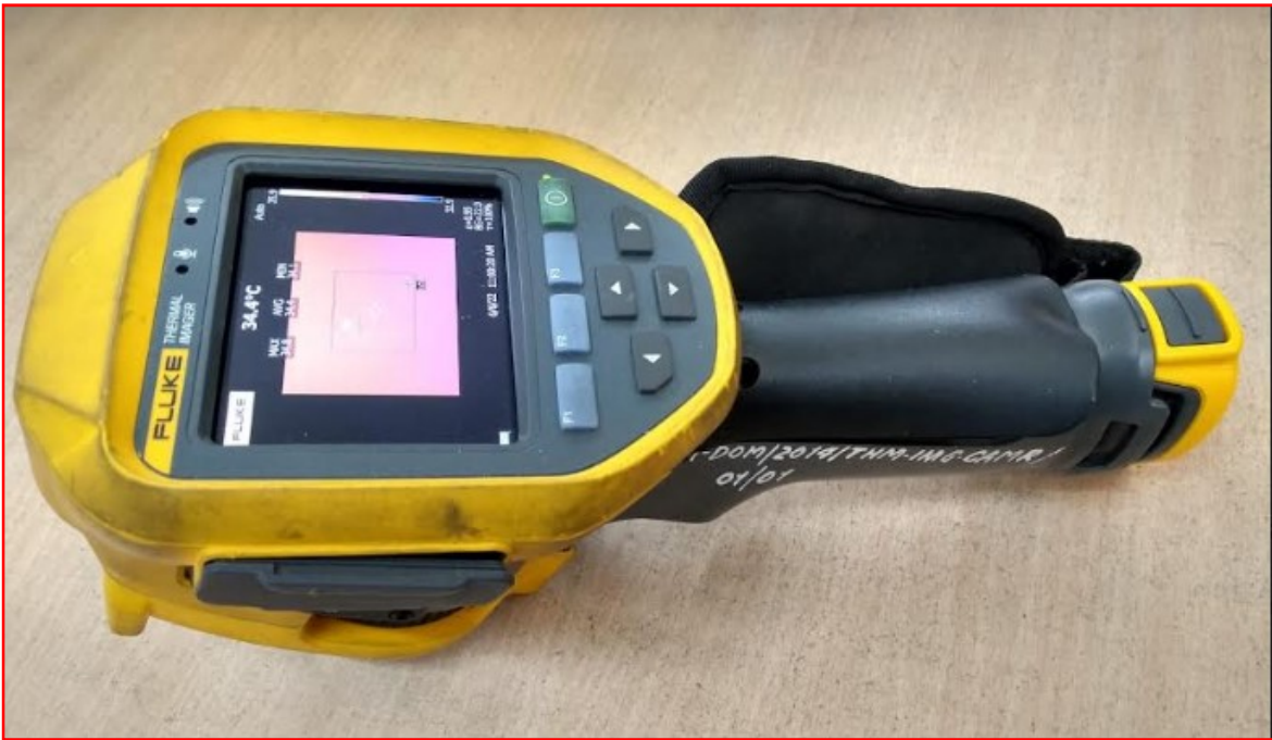
Fig.16: Measurement of tool tip temperature by FLUKE thermal imager
