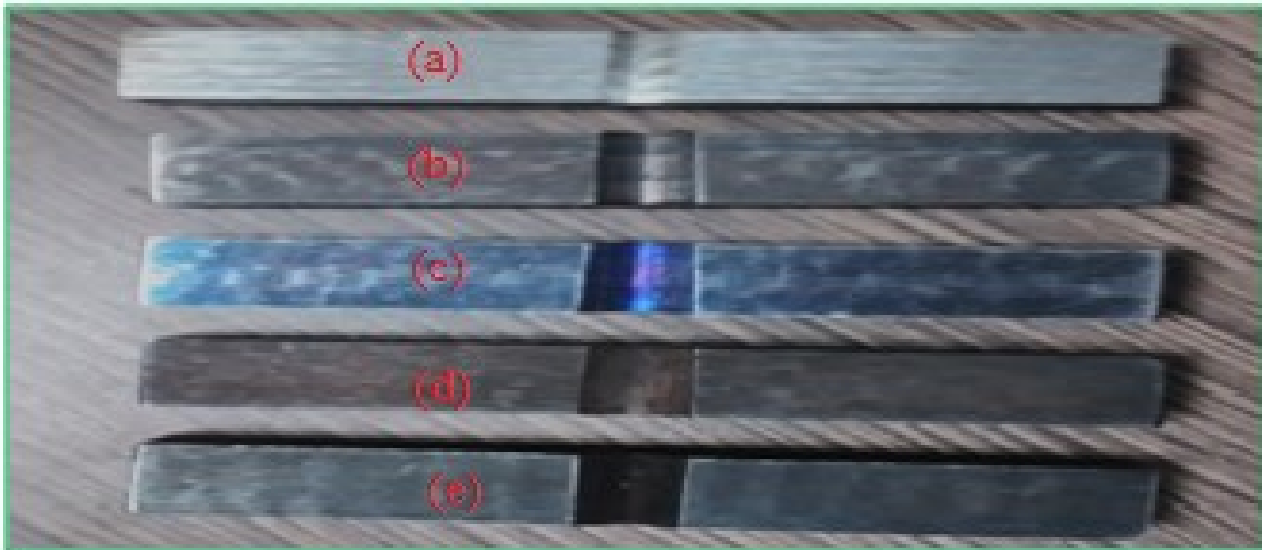
Fig.11: Impact test of EN-36C alloy steel (a) Untempered(b)Tempered at 200°C (c)Tempered at 300°C(d) Tempered at 500°C (e) Tempered at 700°C
