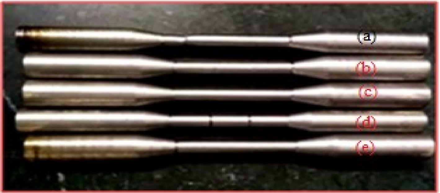
Fig.9: Tensile test specimens (a) Untempered(b)Tempered at 200°C (c)Tempered at 300°C (d) Tempered at 500°C (e) Tempered at 700°C
