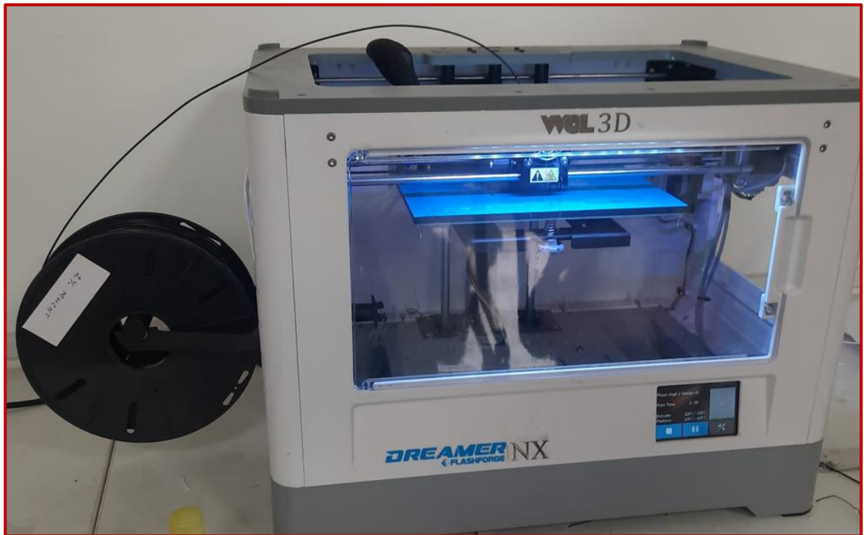
Figure 3.7 Flashforge Dreamer 3D printer used to prepare specimens
