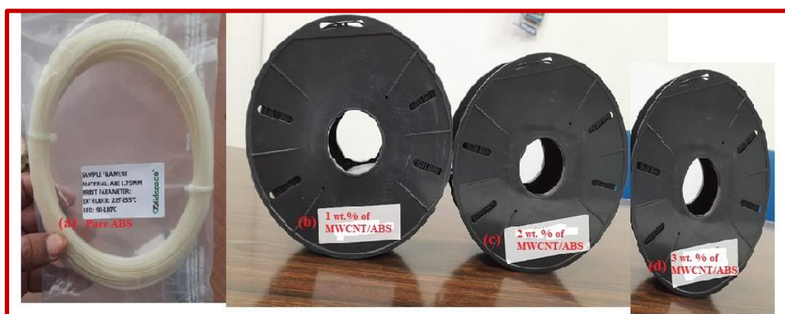
Figure 3.6 Prepared filaments ready to 3 D print (a) Pure ABS, (b) 1wt. % of MWCNT/ABS, (c) 2wt. % of MWCNT/ABS and (d) 3 wt. % of MWCNT/ABS.
