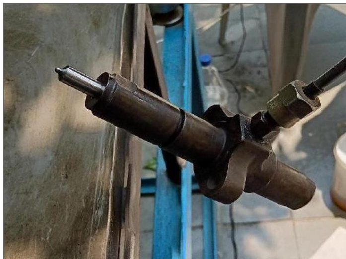
Plate 3.11 Experimental setup Injector used in the setup
