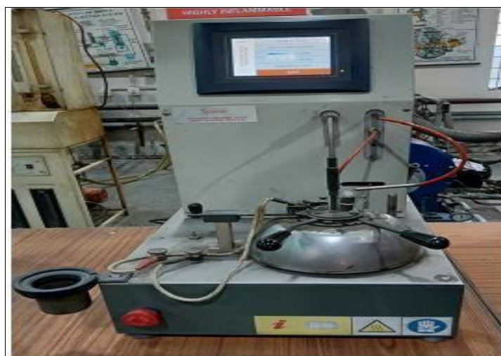
Plate 3.5 Instrument for measuring the flash point
