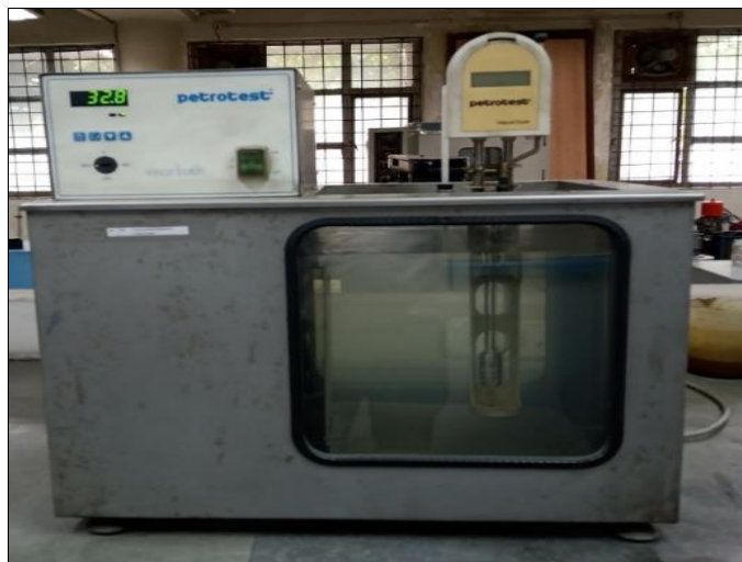
Plate 3.3 Equipment was employed to measure kinematic viscosity
