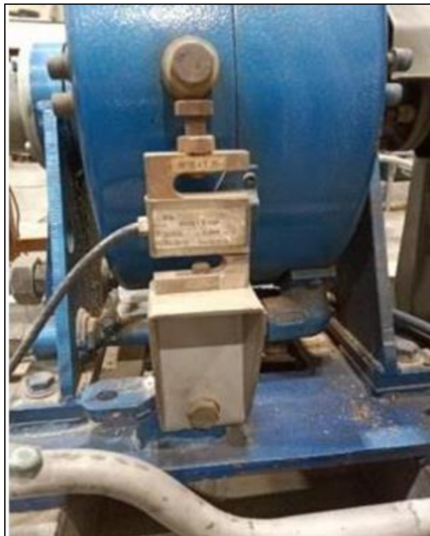
Plate 3.12 Load cell placed on the dynamometer
