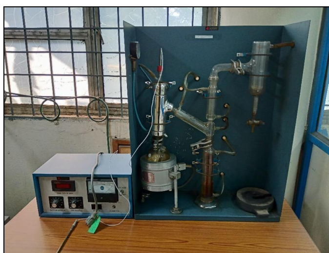
Plate 3.6 Device used to distil the test fuel
