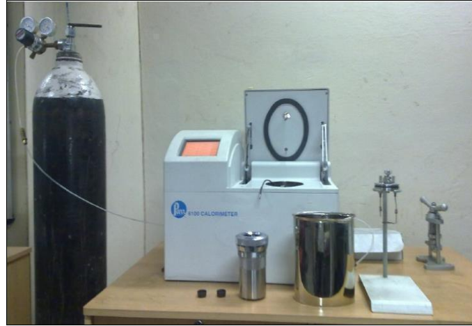
Plate 3.4 Instrument for finding the calorific value
