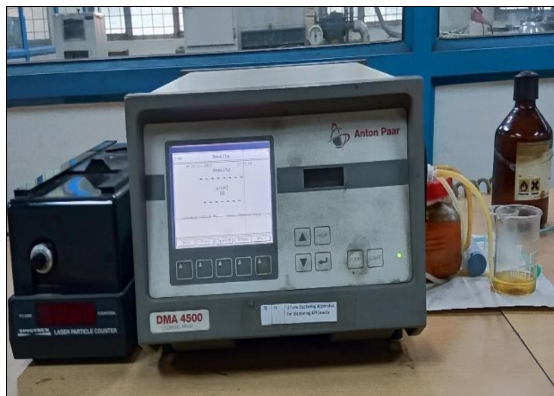
Plate 3.2 The density-finding instrument
