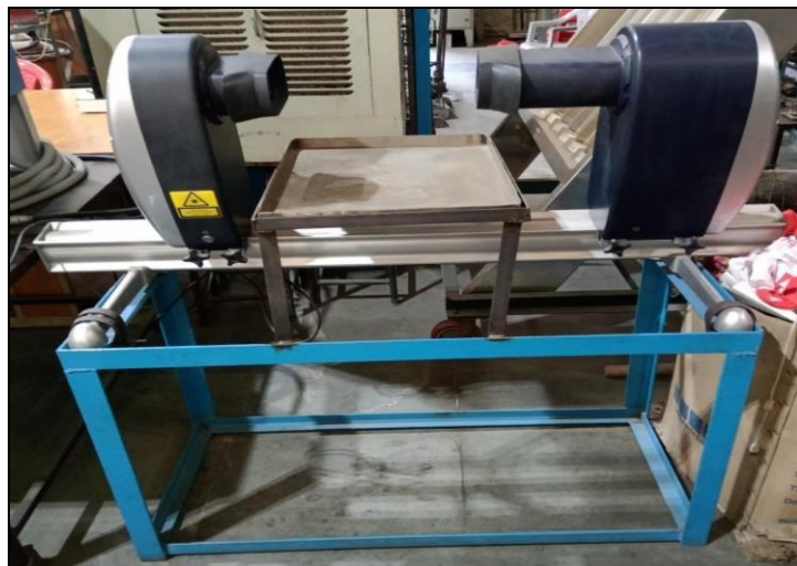
Plate 3.8 Experimental setup for the Malvern Spraytec
