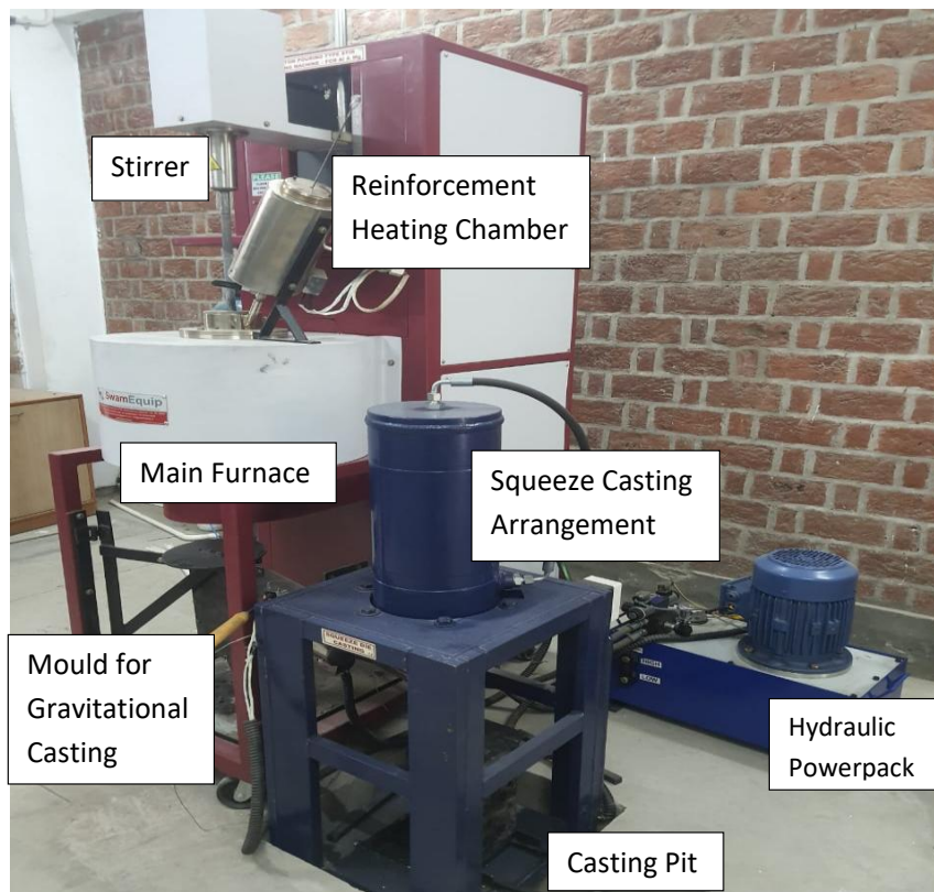
Figure 3.3. Bottom Pouring Type Stir Casting Machine with Squeeze Casting Attachment.
