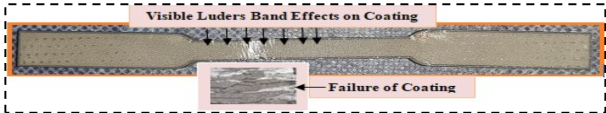
Figure 5.54: Fractured tensile test of 0.9 wt.% rare earth oxides doped sample
