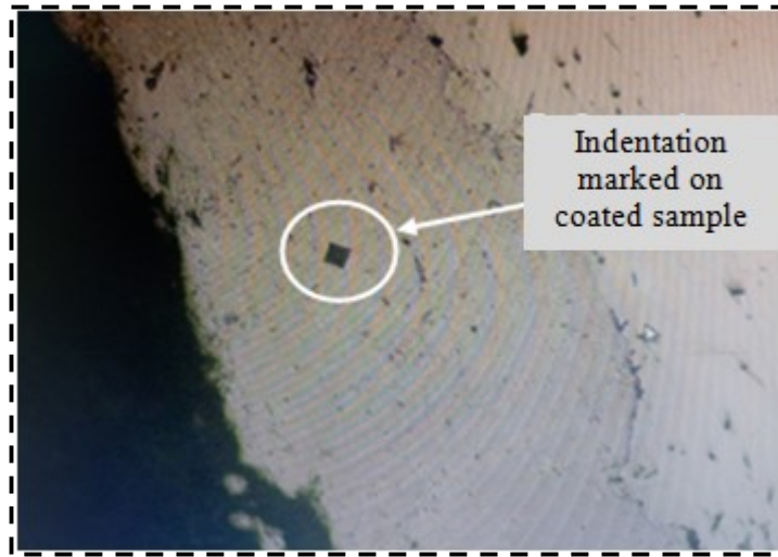
Figure 5.46: Indentation marked on coating
