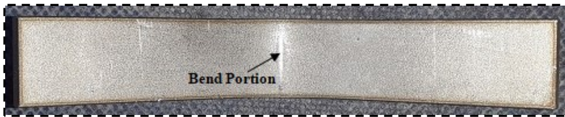
Figure 5.7: Samples of flexural test of the substrate (SS410) after bend test
