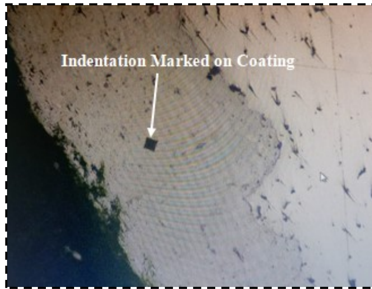
Figure 5.22: Indentation on un-doped coated sample
