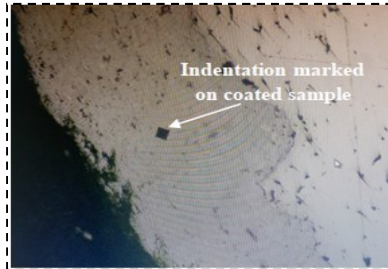
Figure 5.58: Indentation marked on coating for experiment 4 (CpLCE-4)
