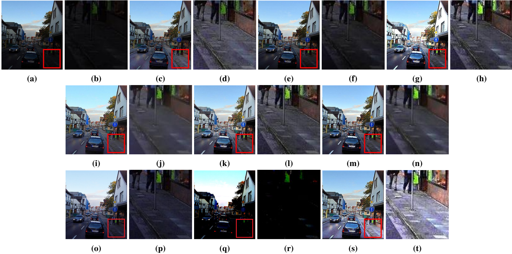
Fig. 3.14: Results of different algorithms on image road. (a) Input image; (b) Patch of (a); (c) NPEA; (d) Patch of (c); (e) PIRE; (f) Patch of (e); (g) LIME; (h) Patch of (g); (i) SRLIME; (j) Patch of (i); (k) LECARM; (l) Patch of (k); (m) LSDD; (n) Patch of (m); (o) Zero-DCE; (p) Patch of (o); (q) CSDGAN; (r) Patch of (q); (s) Proposed method; (t) Patch of (s).
