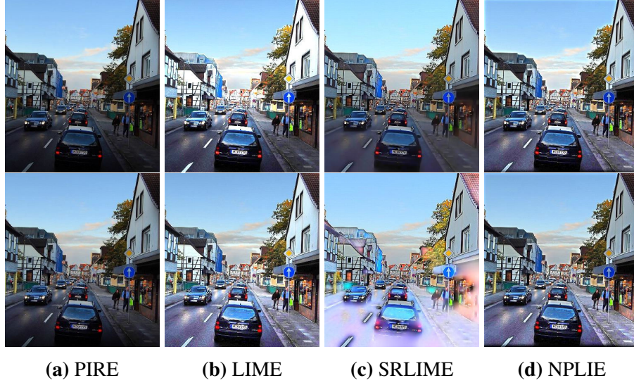
Fig. 3.10: Assessment of proposed adaptive illumination adjustment. Top row shows the results with traditional gamma (for illumination adjustment on various approaches), and bottom row shows the results with proposed adaptive illumination adjustment on various approaches.
