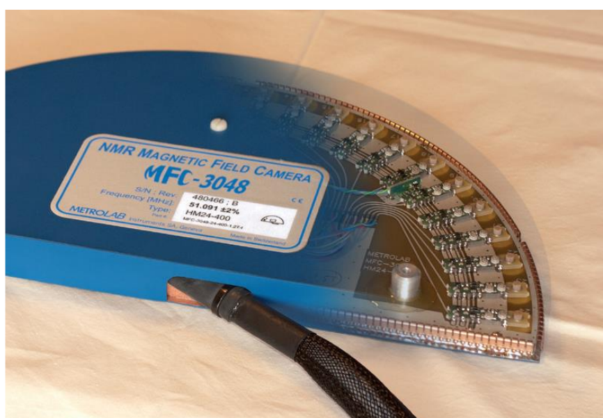
Figure 5.35 The NMR half-moon camera with an overlap showing the PCB where 18 individual NMR probes are arranged to form a circle.
