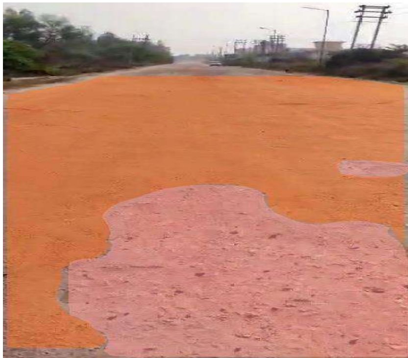
Fig 3.4 Segmentation Example of Road and Pothole
