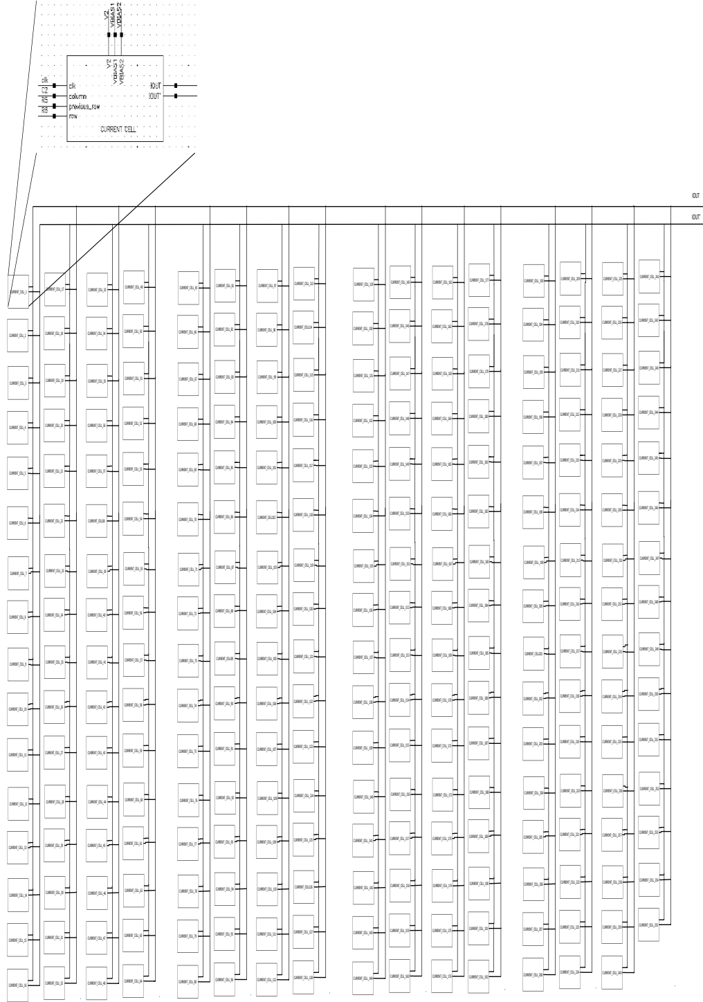
Fig.3.2: Unary current cell Array Schematic
