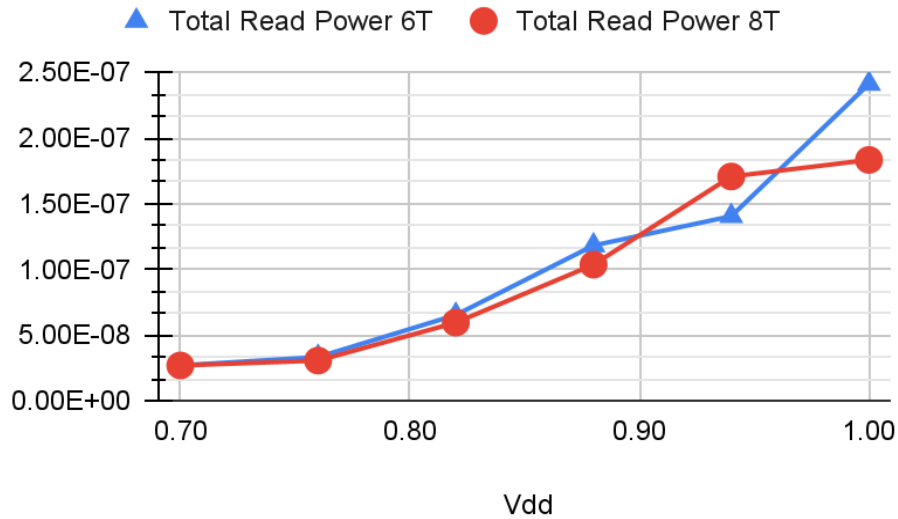
Fig. 5.7. Line Chart for Total Read Power vs Vdd
