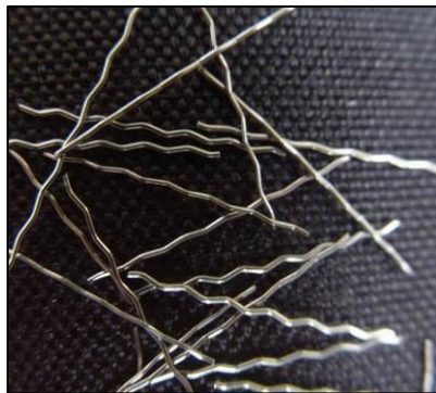
Figure 1.6 Crimped steel fibres
