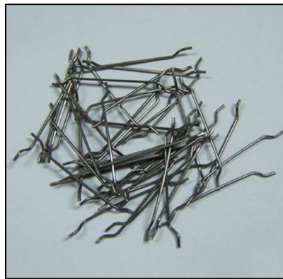
Figure 1.7 Hooked end steel fibres
