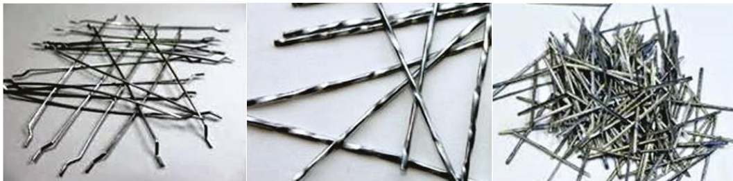
Figure 1. 1 Steel fibres – Hooked end, twisted and straight [2]
