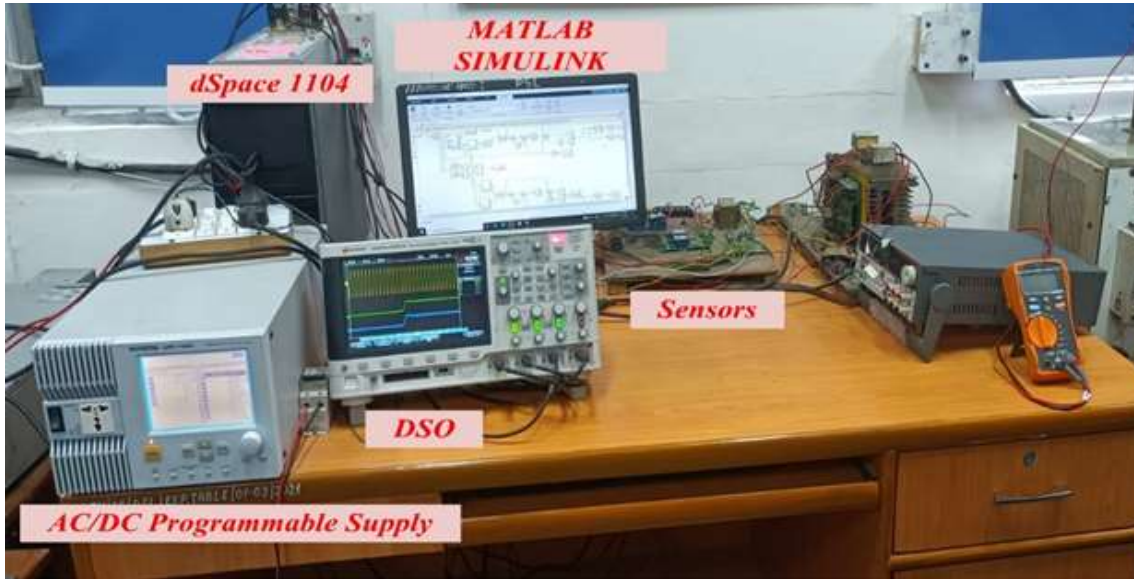
Fig. 7. 22 Photograph of the setup for testing of grid synchronization schemes
