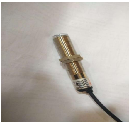
[Fig 4.2: Diffused photoelectric Sensor]
