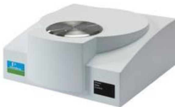
Figure 2.5: Thermo-Gravimetric Analyser (Perkin-Elmer TGA4000)
