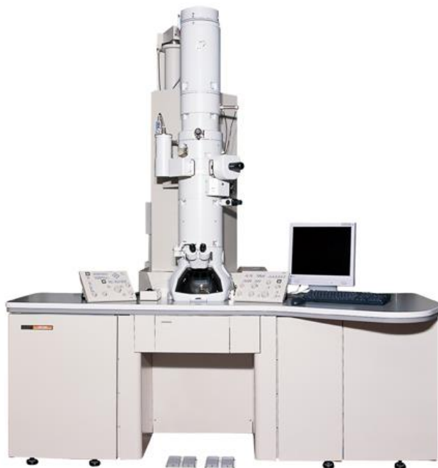
Figure 2.2: Transmission Electron Microscopy (Jeol/JEM 2100)
