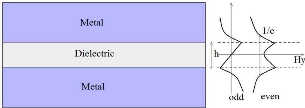
Figure 3. 7 a) SPP at the multilayer MIM Interface b) Even and odd modes
