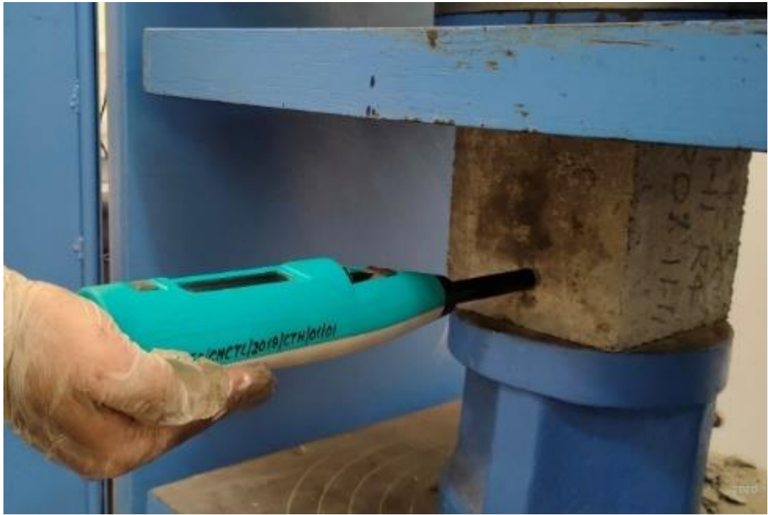
Fig. 3.27 Rebound hammer testing of the cube for the compressive strength test
