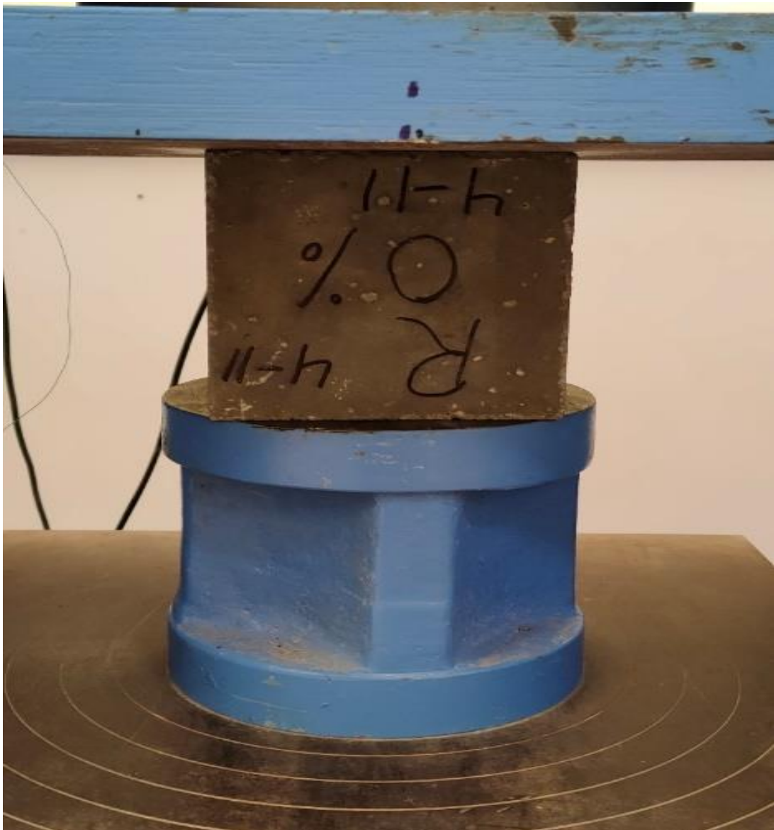
Fig. 3.22 Testing setup for compressive strength in the CTM
