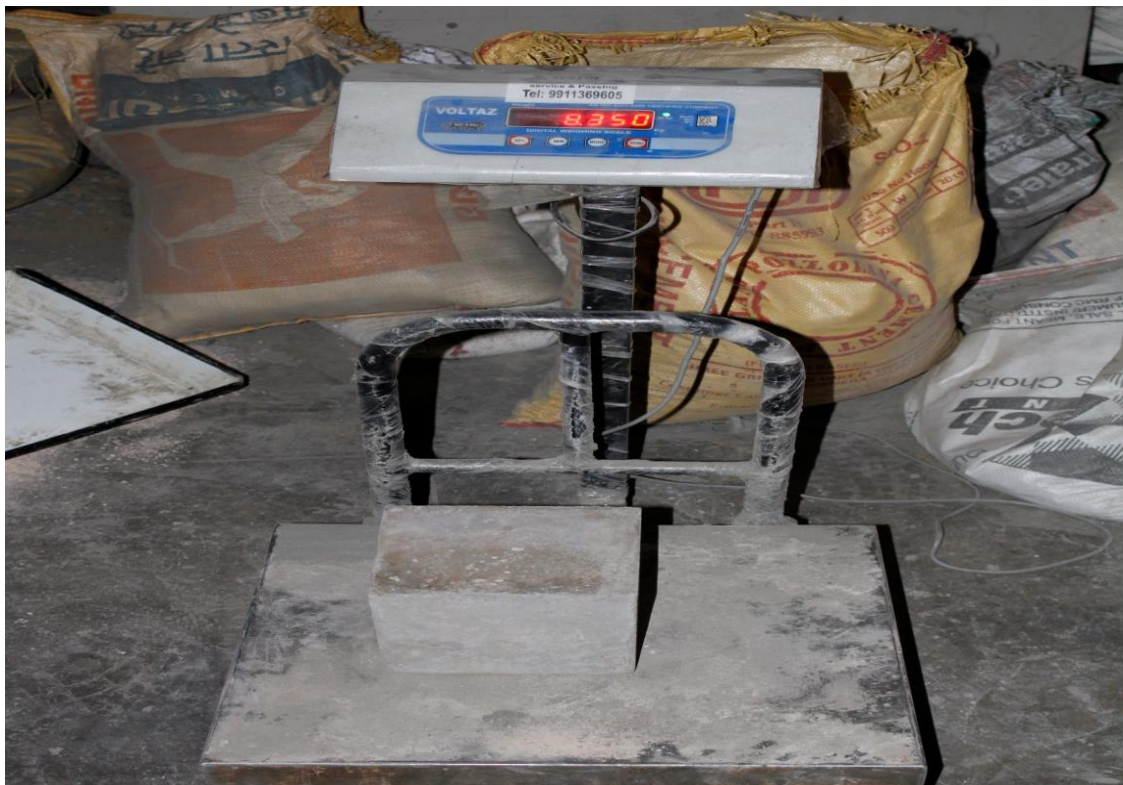
Fig. 3.21 Digital weight machine for finding density by weight of the cube
