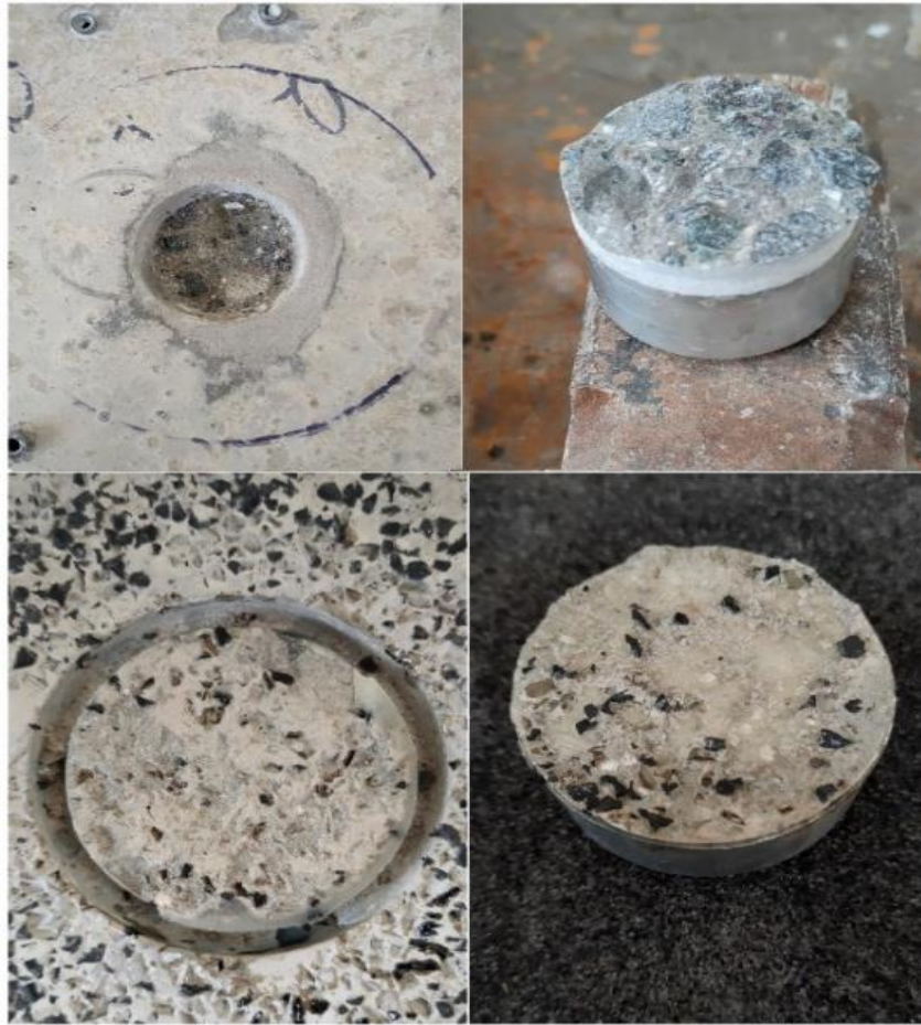
Fig. 4.14 Failure pattern of standard and RuC in pull-off test
