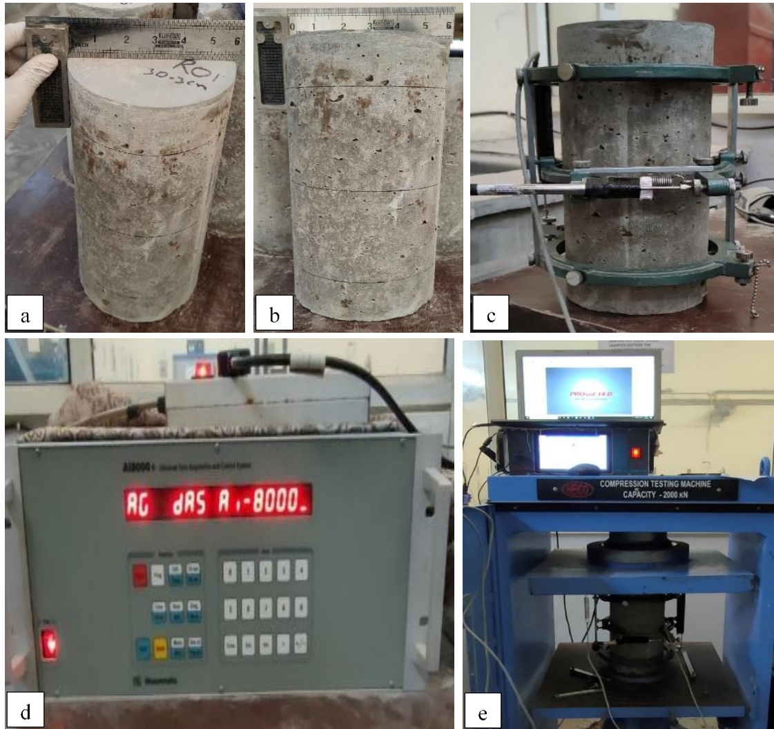
Fig. 3.26 (a) Capping of the cylinder specimen, (b) Marking of the cylinder specimen, (c) Arrangements of extensometer and LVDTs, (d) Data acquisition system for LVDTs, (e) Testing setup of the cylinder for modulus of elasticity and poisson's ratio
