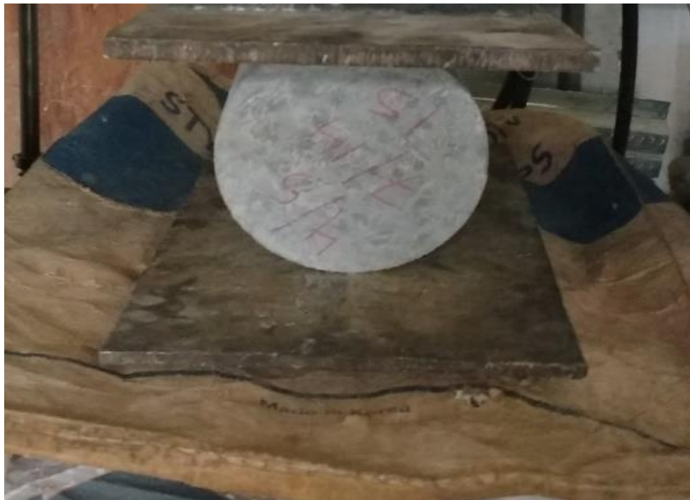
Fig. 3.23 Testing setup for splitting tensile strength of concrete
