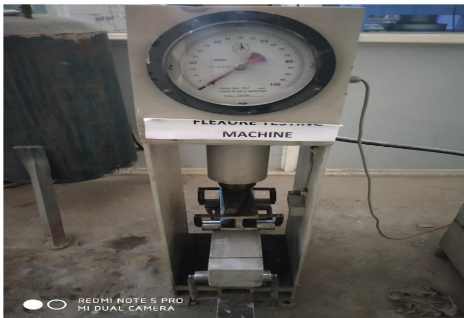
Fig. 3.25 Testing setup for flexural strength of concrete
