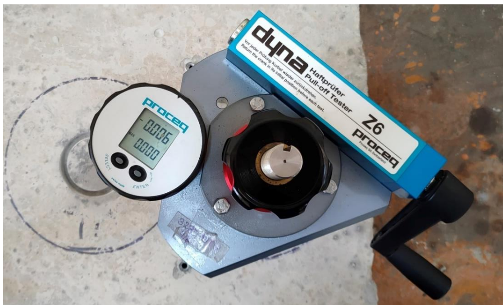
Fig. 3.33 Top view of the pull-off tester with a digital recorder on slab specimen
