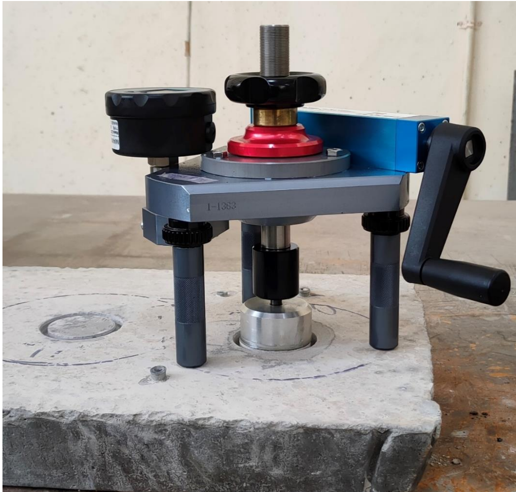
Fig. 3.32 Side view of the pull-off tester on slab specimen
