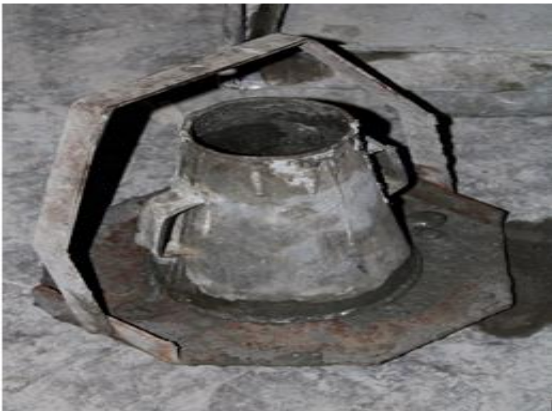
Fig. 3.20 Apparatus for slump test
