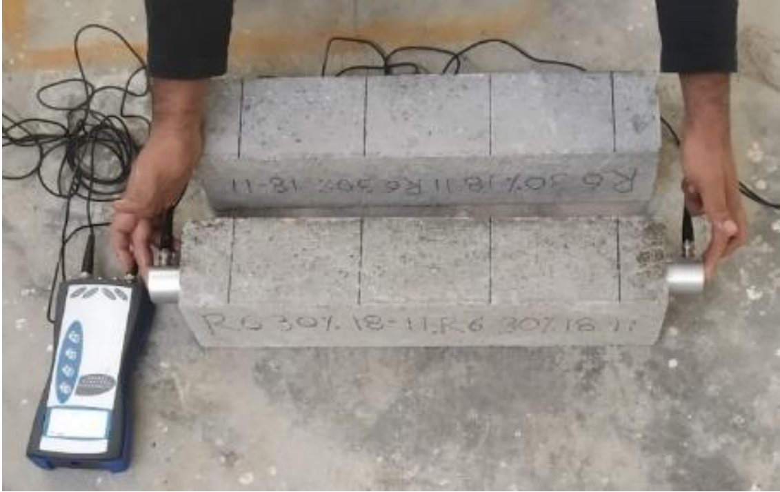
Fig. 3.28 Ultrasonic pulse velocity testing setup of standard concrete and RuC
