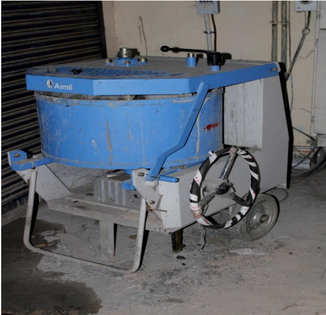
Fig. 3.18 Pan mixture in the laboratory
