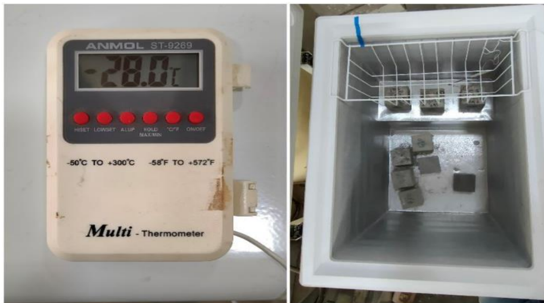
Fig. 3.35 Testing setup for freeze-thaw cycles of RuC specimens
