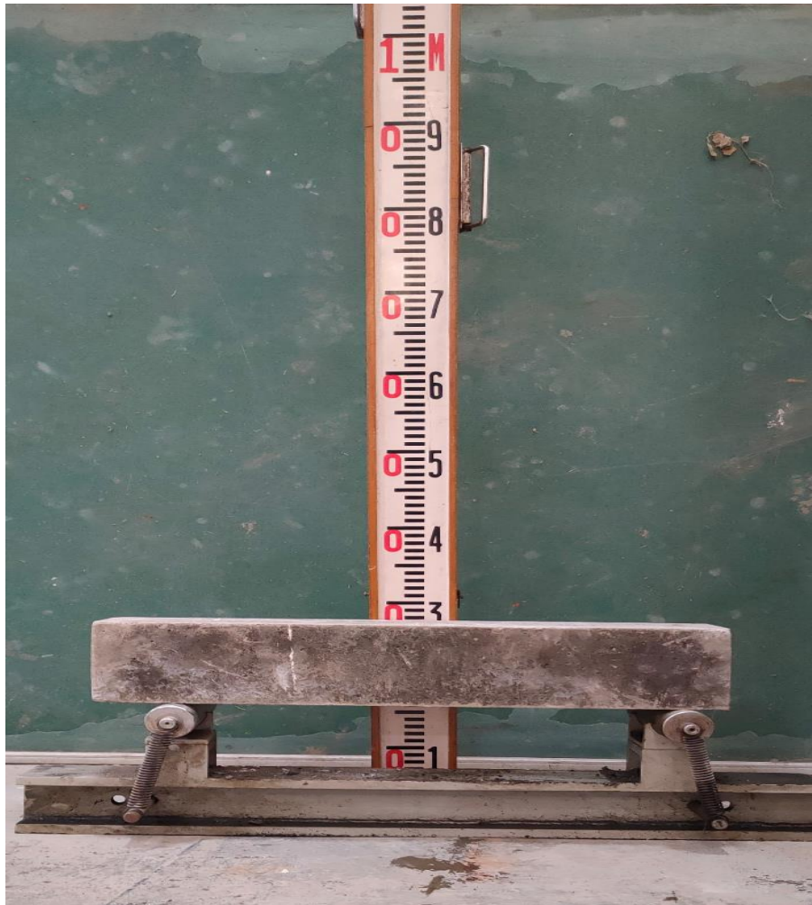
Fig. 3.29 Testing setup for impact energy by the flexural loading of standard and RuC
