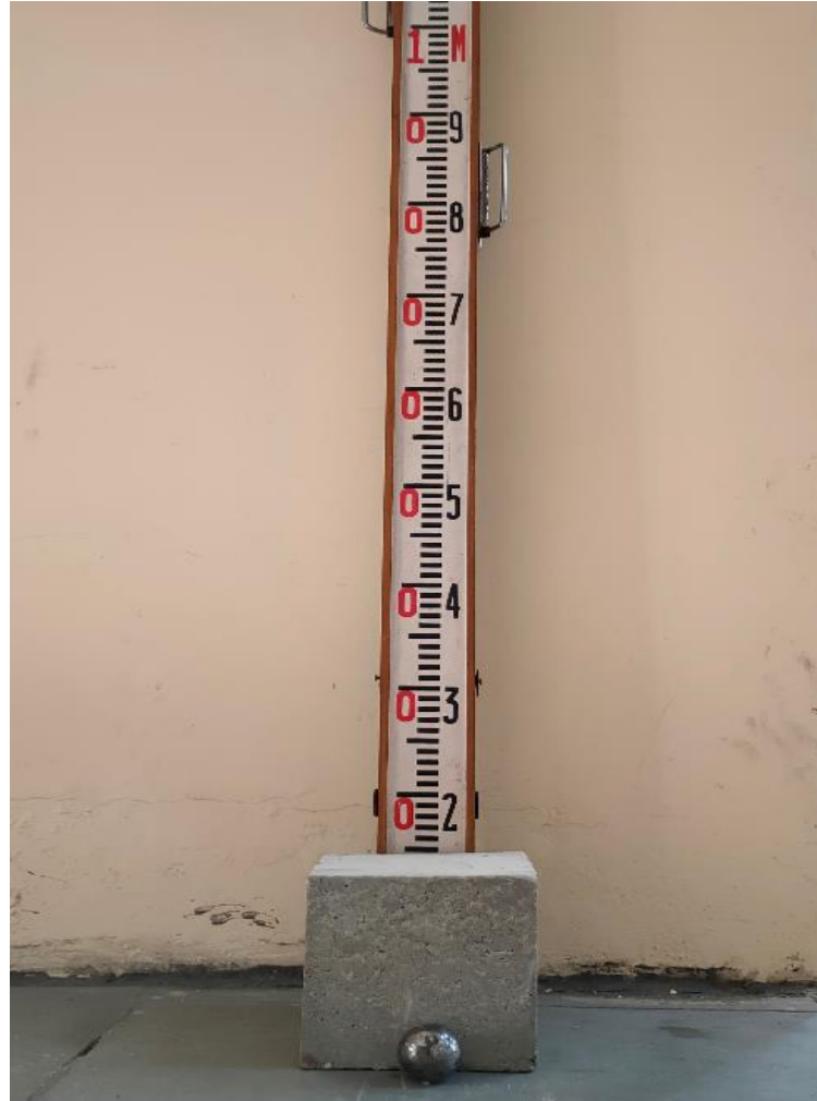
Fig. 3.30 Testing setup for impact resistance by rebound test of standard and RuC
