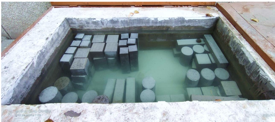
Fig. 3.19 Curing of concrete specimens in clean water
