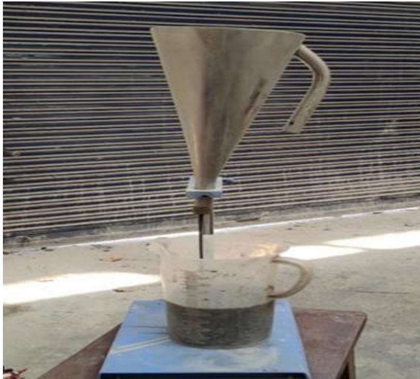
Fig. 3.3 Testing setup of marsh cone apparatus
