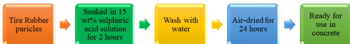
Fig. 3.10 Sequence of surface treatment of the rubber crumbs
