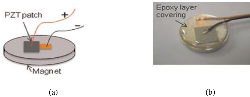
Figure 2. 9 Reusable setup (Na et al. 2012)
