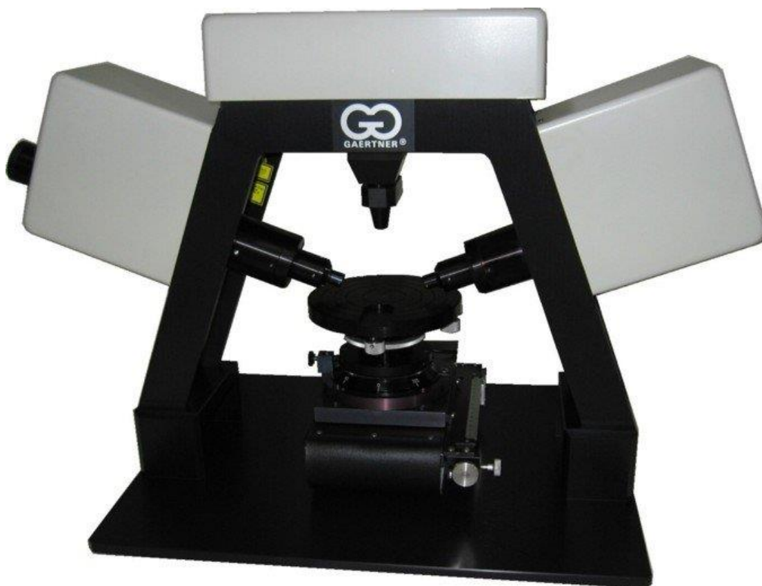
Figure 2.9. Photograph of the ellipsometer used to examine the surface quality of HgCdTe samples.
