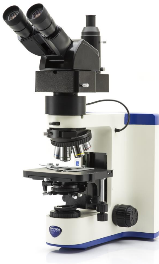
Figure 2.10. Nomarski microscope used for the inspection of HgCdTe samples surfaces.
