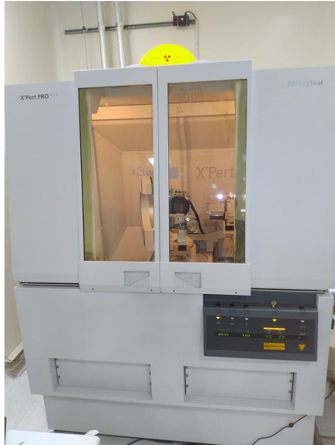
Figure 2.3. Photograph of X-ray diffraction system of PANalytical B.V.-X'Pert PRO MRD (Material research diffractometer).
