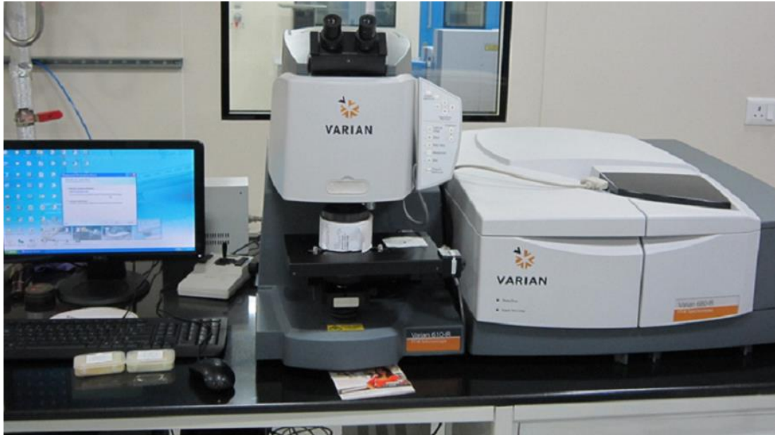
Figure 2.7. FTIR spectrometer used for measuring the reflectance of thermally grown ARC film stacks ( \text{YF}_3/\text{ZnS}/\text{YF}_3/\text{ZnS}/\text{CdZnTe} -HgCdTe).
