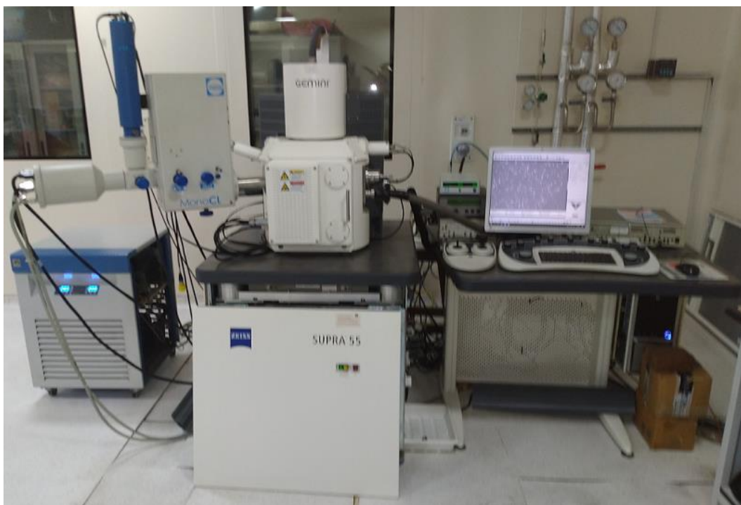
Figure 2.5. Photograph of SEM system supported with EDX spectrometer.
