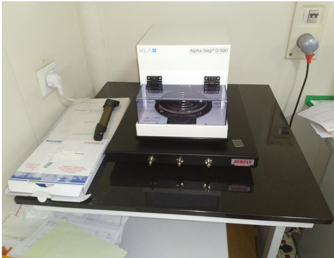
Figure 2.8. Photograph of the surface profiler (Model: Alpha Step* D-500) used for measuring the thicknesses of thin films.
