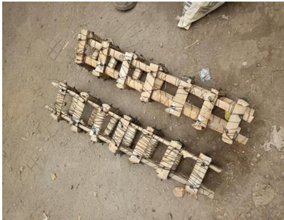
Fig. 3.10 Reinforcement Detailing of Bamboo Concrete Beam
