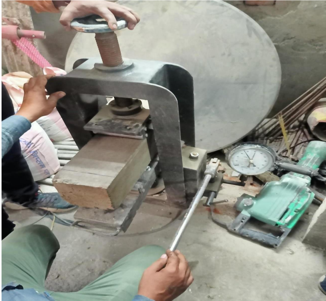
Fig. 3.11 Flexural strength Test Setup for Bamboo Concrete Beam
