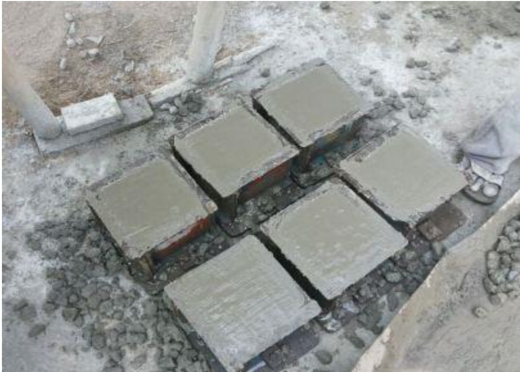
Fig. 3.4 Concrete Samples for Compressive Strength Test
