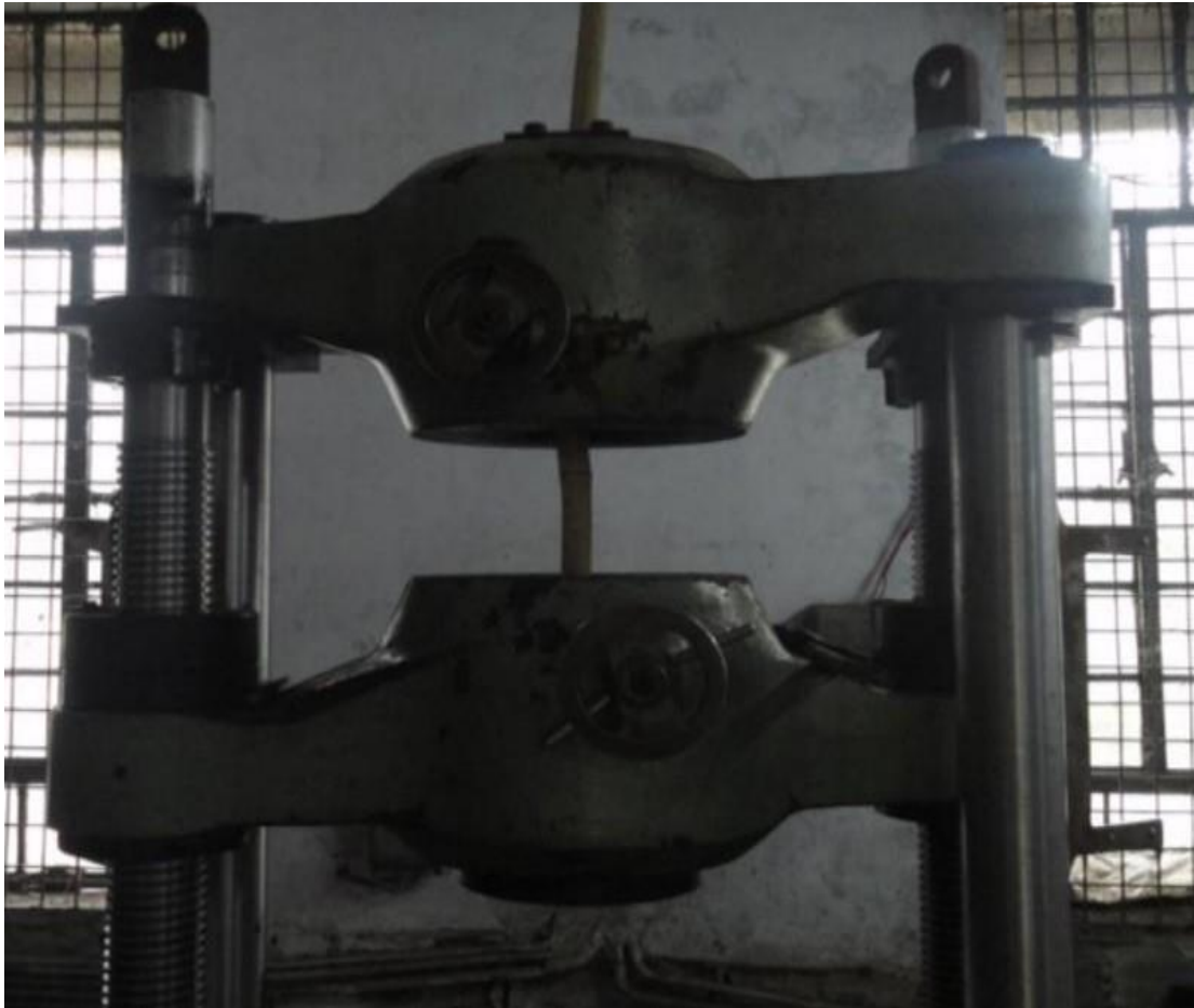
Fig. 3.5 Tensile Strength Test of Bamboo Stick
