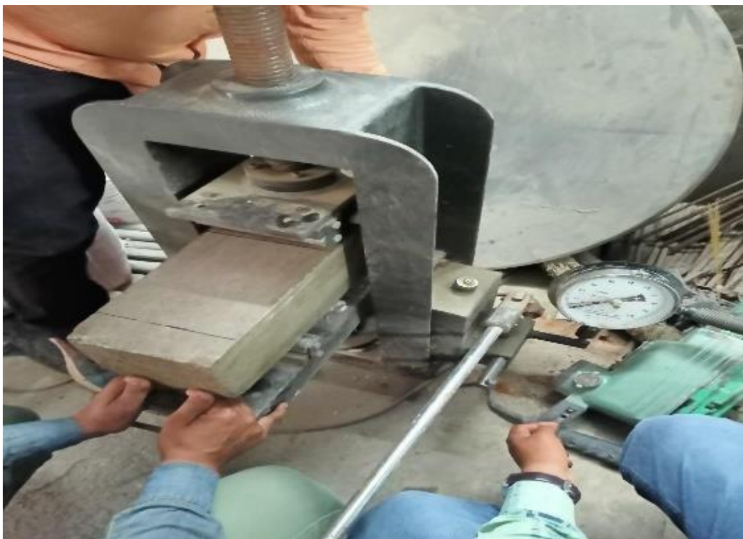
Fig. 3.9 Test Setup for flexural strength test of RCC Beam
