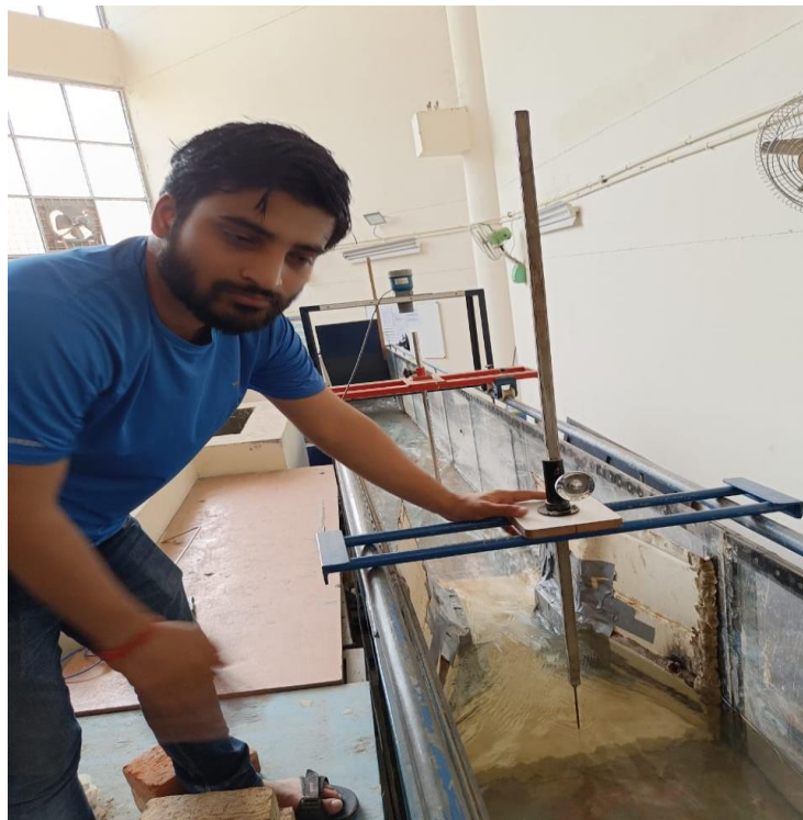
Figure 3.9 Measurement of depth
