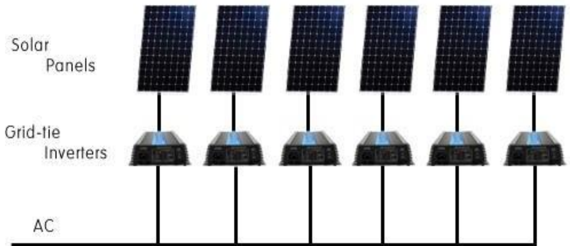
Fig 2.3.2: Inverter Connection in parallel
