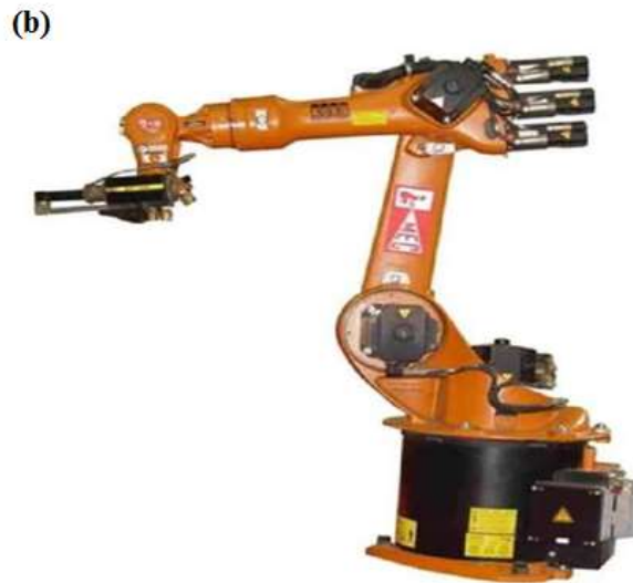
Figure 1.2 schematic diagram of the (a) HVOF spray process [25] and (b) Thermal Spray Robot [27]
