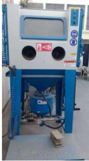
Figure 2.7 systematic diagram of pressure blaster of HVOF thermal spray system
