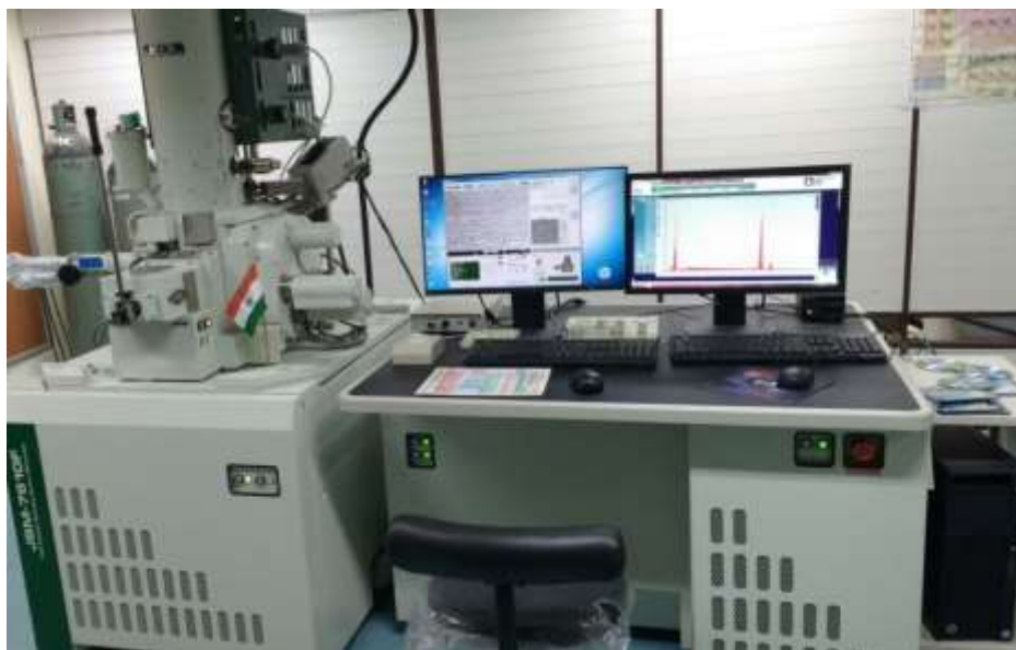
Figure 4.1 Systematic diagram of FESEM attached with EDS
