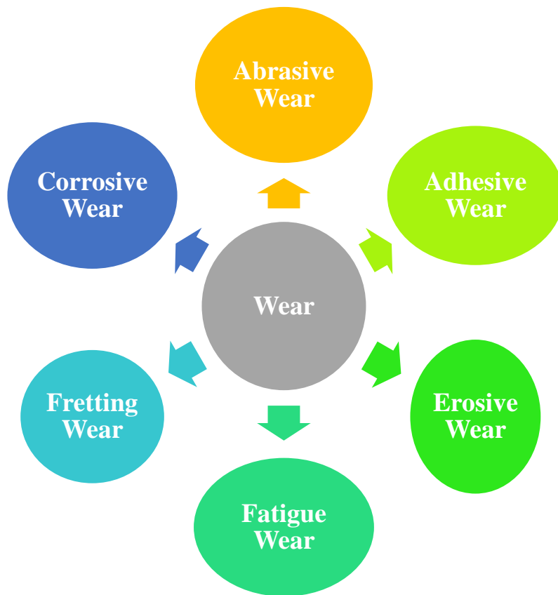
Fig 1.6 systematic sketch of types of wear
