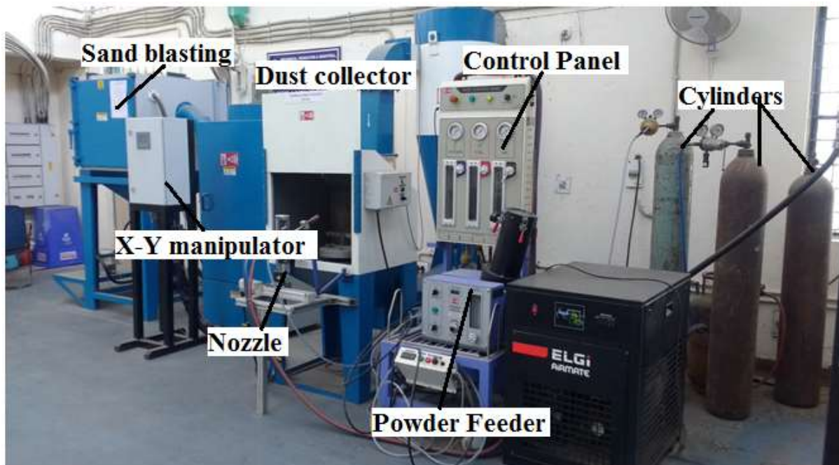
Figure 2.6 systematic diagram of HVOF thermal spray system
