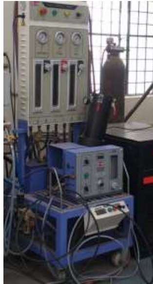
Figure 2.11 systematic diagram of powder feeder of HVOF thermal spray system
