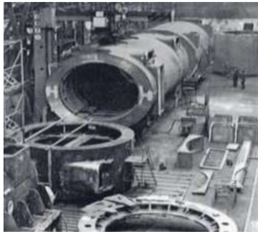
Figure-1.1: Submerged arc welding for circumferential joint in large fabrication (Houldcroft, 1989)
