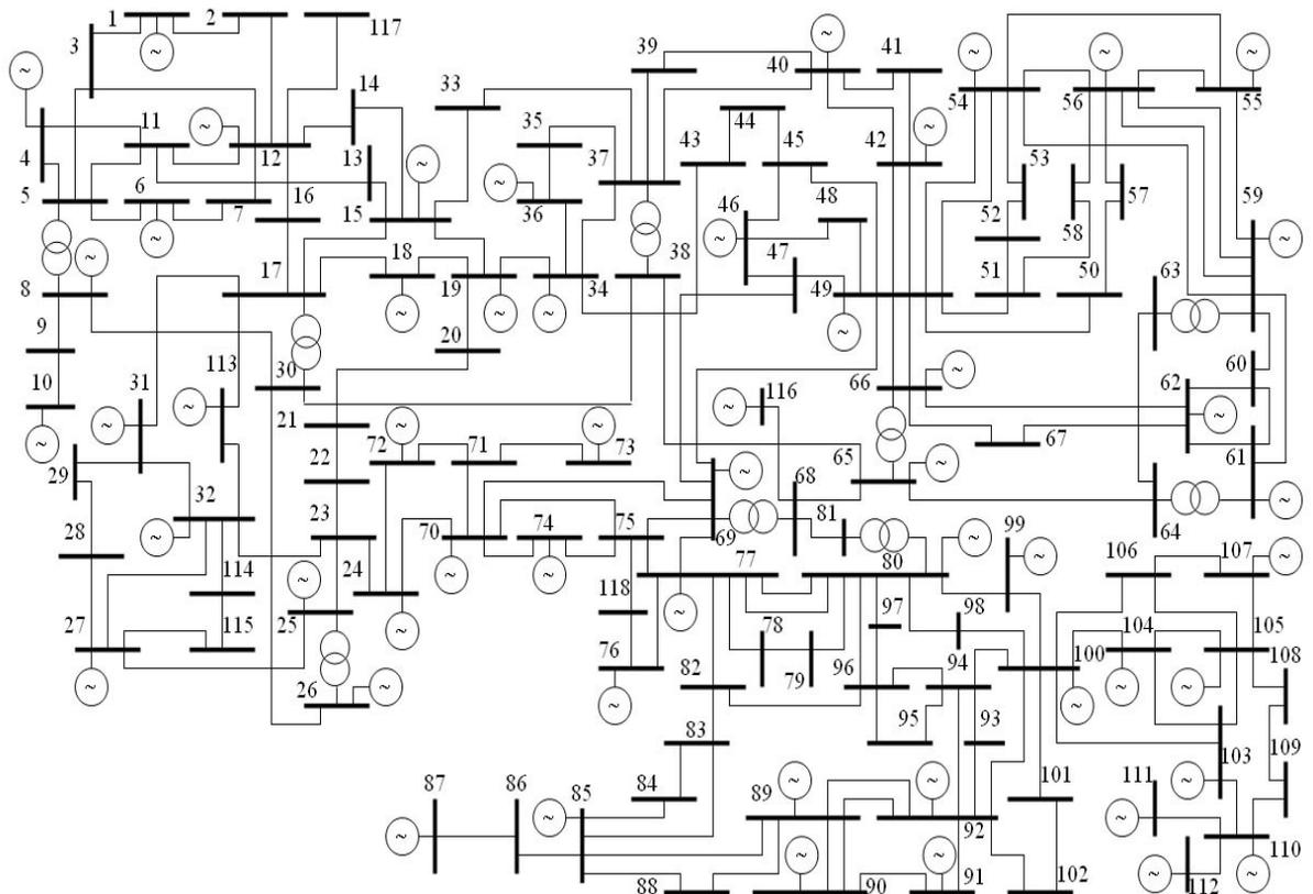
Figure D. Single line diagram of IEEE-118 Bus Test System
