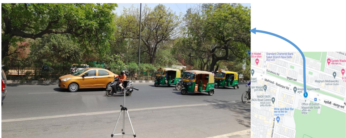
Figure 3. 9. Noise monitoring at Mehrauli Badarpur Road
