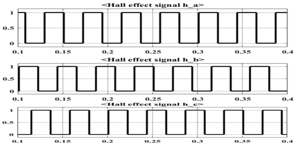
Fig.3.5: Hall-sensor waveform
