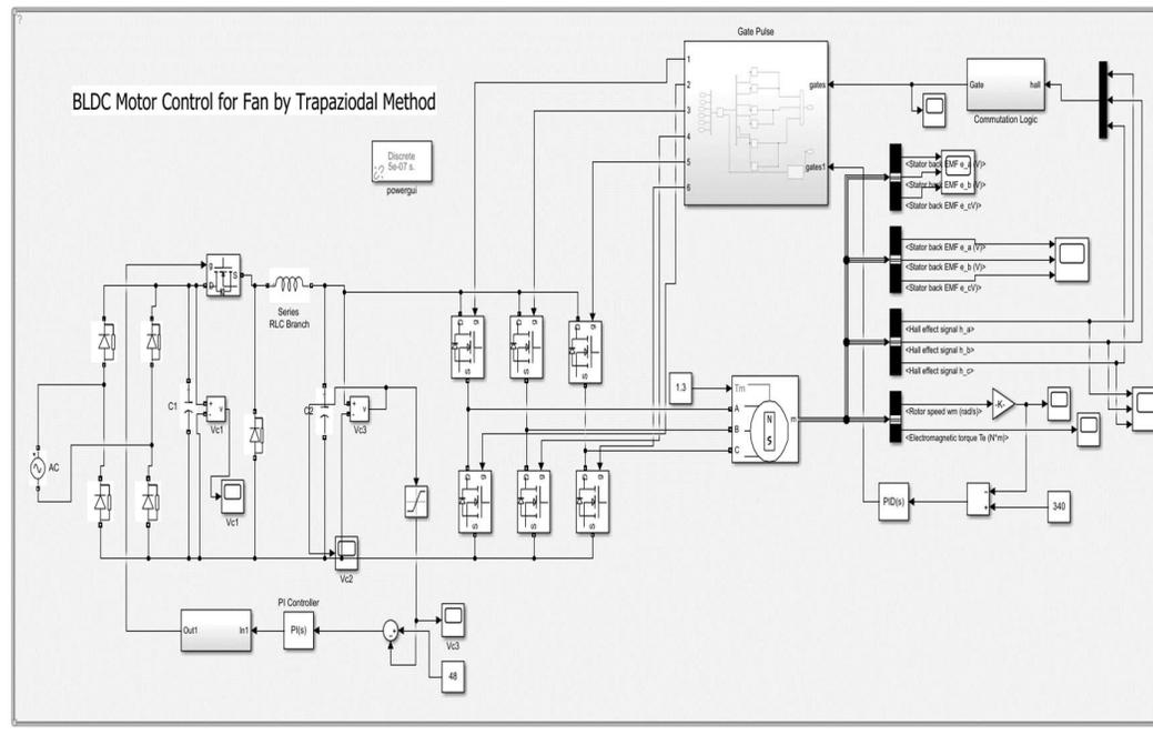
Fig.4.5: Simulation of BLDC motor control by Trapezoidal Method
