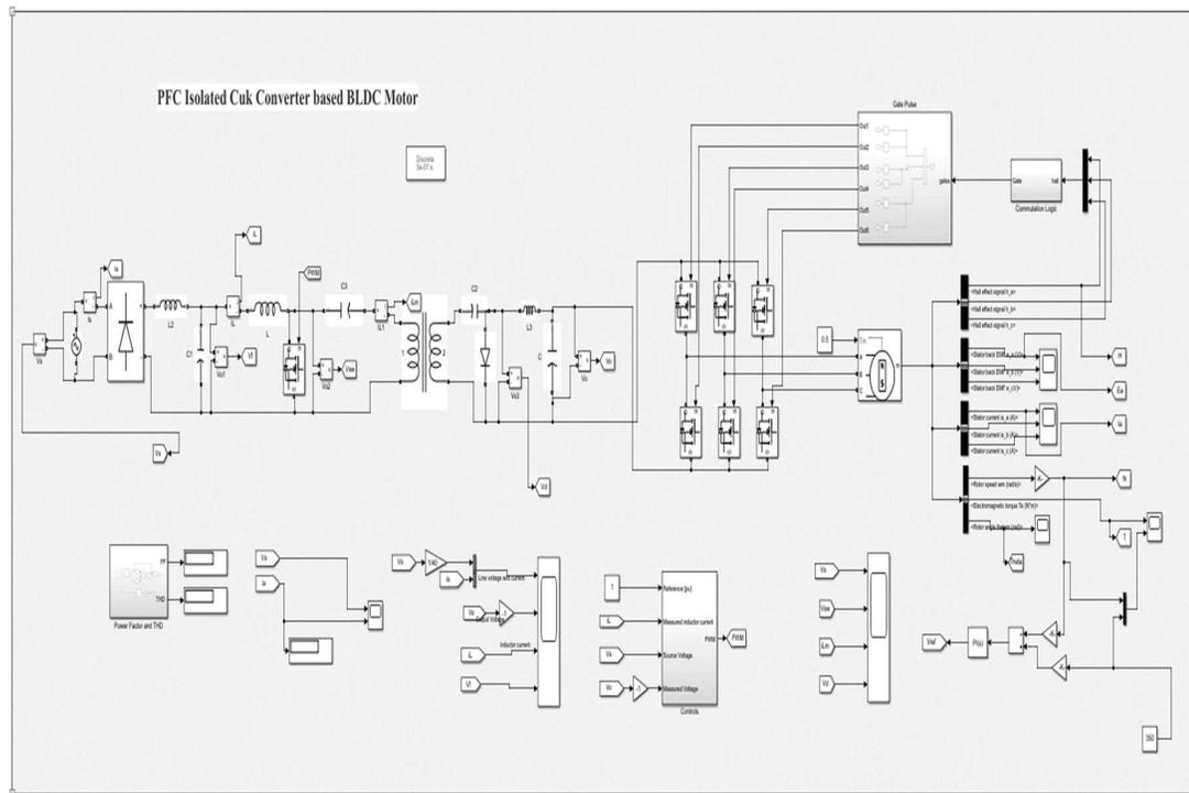
**Fig.5.2:** Simulation of PFC Isolated Cuk Converter based BLDCM
