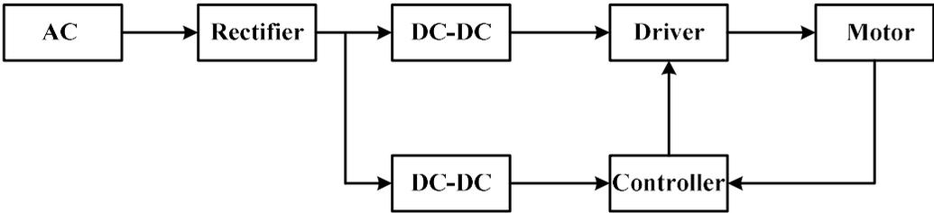
Fig.4.1: Block Diagram of working of BLDC by AC supply
