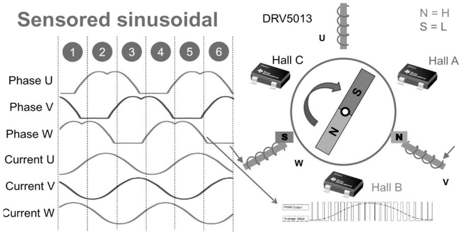
Fig.1.8: Sensored Sinusoidal Control
