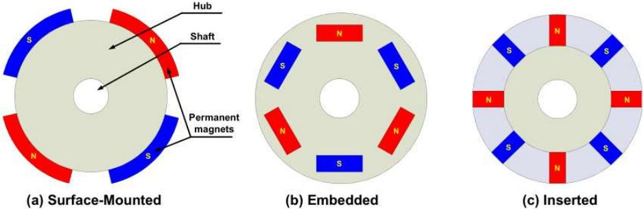
Fig.1.2: Rotor Magnets Cross-Sections
