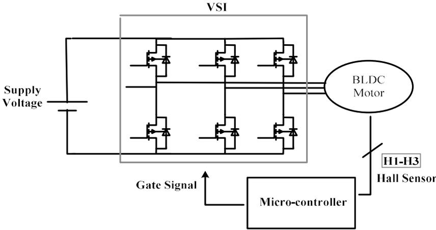
Fig.3.1: Circuit diagram of the 3-phase BLDC motor.
