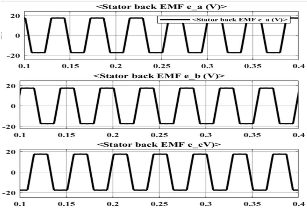
Fig.3.3: BEMF waveforms
