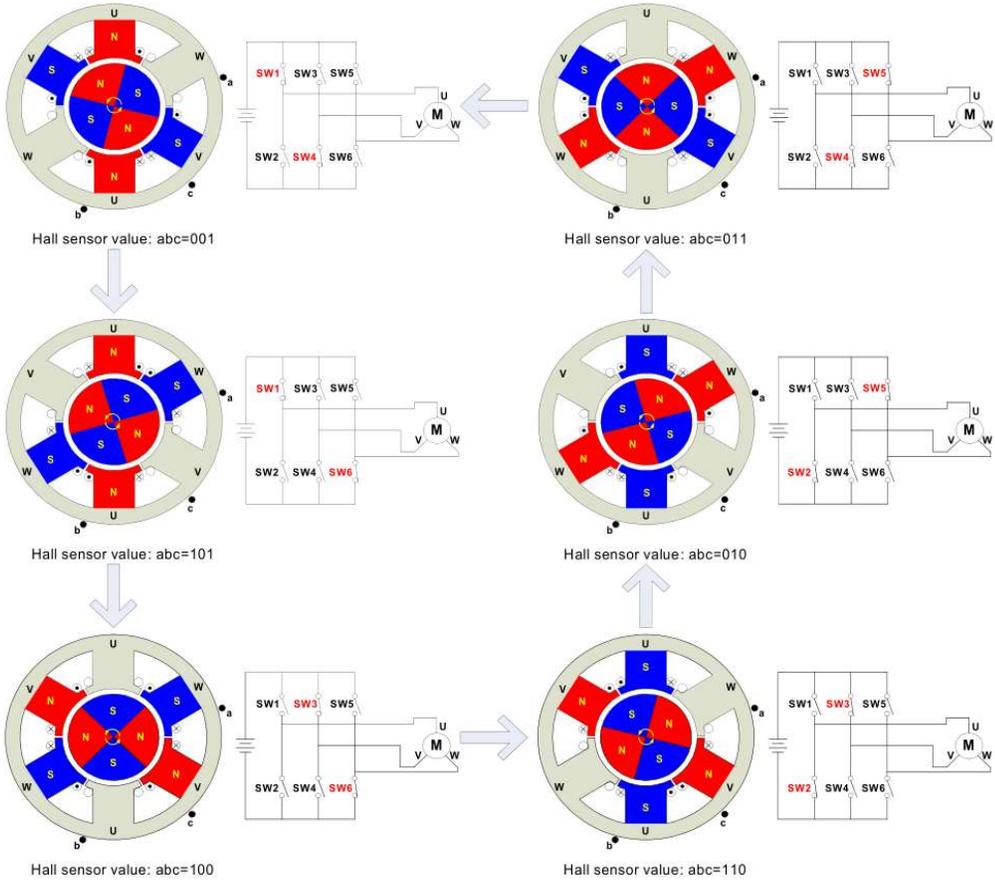
Fig.1.4: Three-Phase BLDC Motor working
