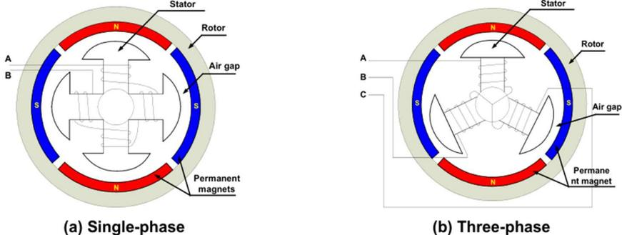
Fig.1.1: BLDC Stator Diagrams
