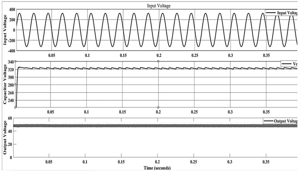
Fig 4.6: Input supply, capacitor voltage and converter output voltage
