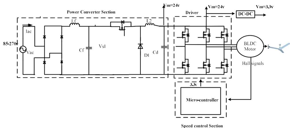
Fig.4.3: Circuit diagram of working of BLDC Motor FAN
