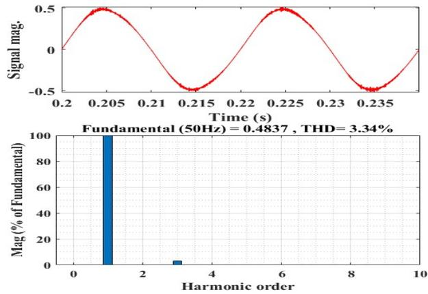
Fig. 5.9: THD in supply current (RMS) at a supply voltage of 270V.
