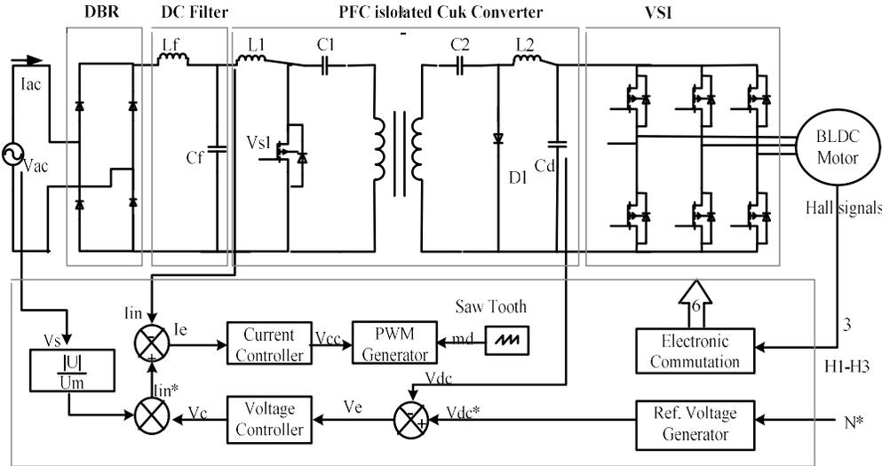
Fig.5.1: A BLDC Motor drive fed by a PFC Isolated Cuk converter in CCM (using a current multiplier approach).
