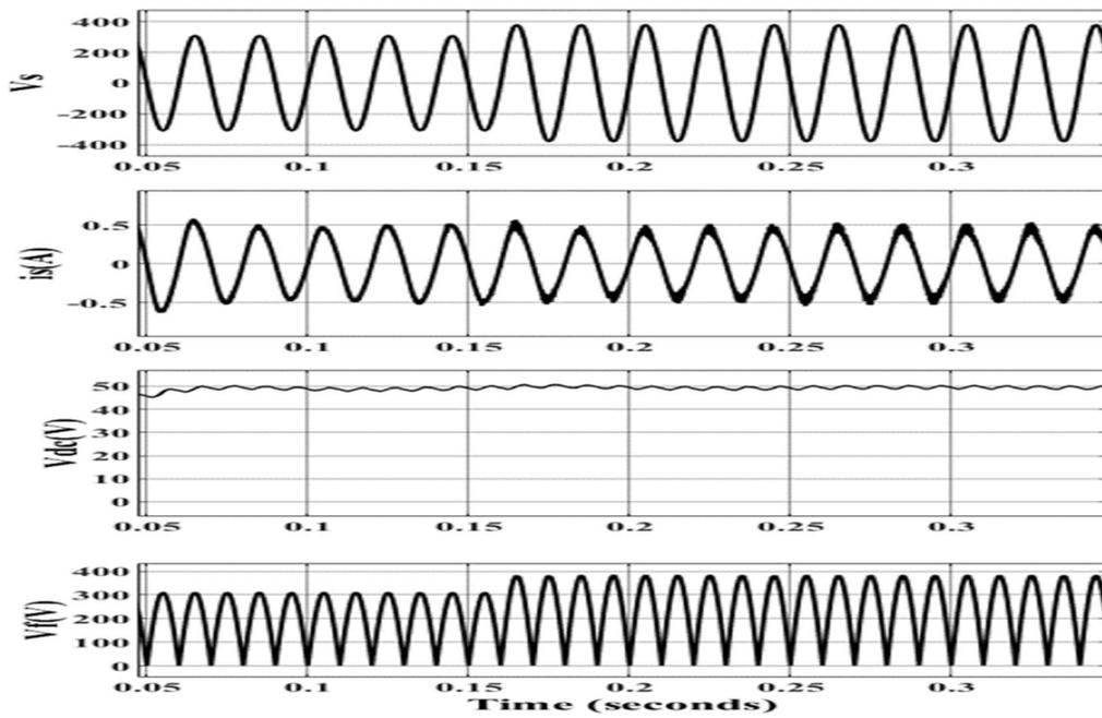
Fig5.7: Input Voltage, Input current, Dc link voltage and capacitor filter voltage at input supply voltage from 220V to 270 V and converter output voltage of 48V
