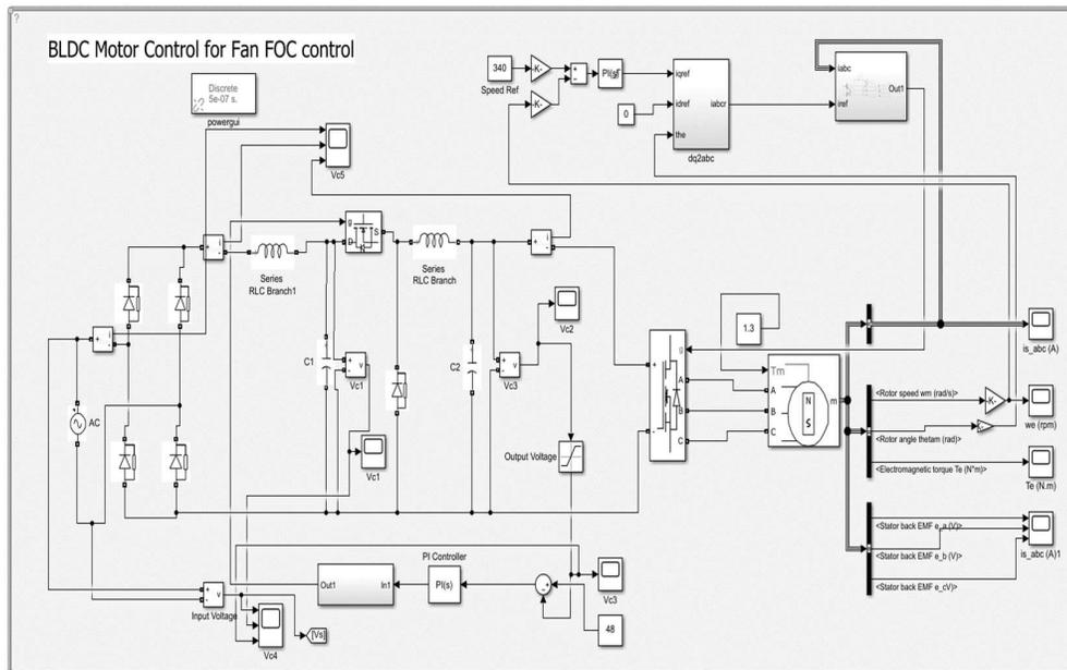
Fig.4.9: Simulation of BLDC motor control by FOC Method
