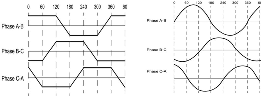
Fig 1.3: Trapezoidal and Sinusoidal stator windings
