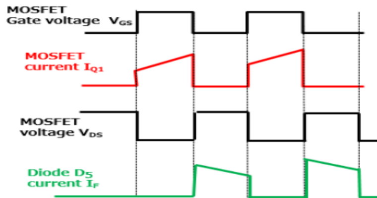
FIGURE 2.8 TYPICAL WAVEFORMS IN CONTINUOUS CONDUCTION MODE (CCM) MODE
