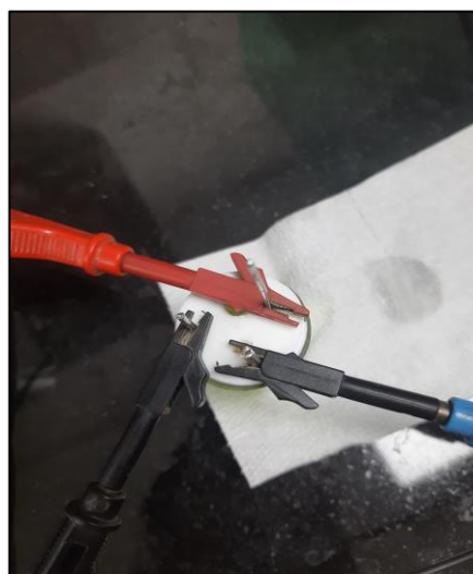
Figure 24: Electrochemical cell containing GOx/PANI/ITO as working electrode, Platinum as counter electrode and Ag/AgCl as reference electrode, and Top view of electrochemical cell electrodes.
