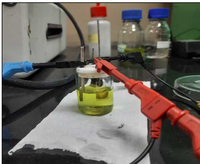
Figure 24: Electrochemical cell containing GOx/PANI/ITO as working electrode, Platinum as counter electrode and Ag/AgCl as reference electrode, and Top view of electrochemical cell electrodes.
