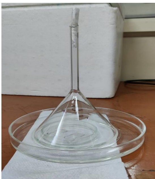
Figure 22: Immobilization of GOx onto PANI/ITO electrode in Humid Chamber.
