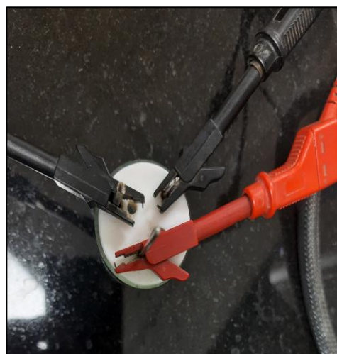
Figure 17: Different electrodes of electrochemical cell (Working- ITO, Reference –Ag/AgCl and Counter- Platinum).
