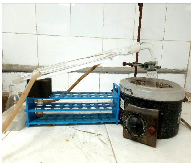
Figure 15: Steam distillation of aniline.
