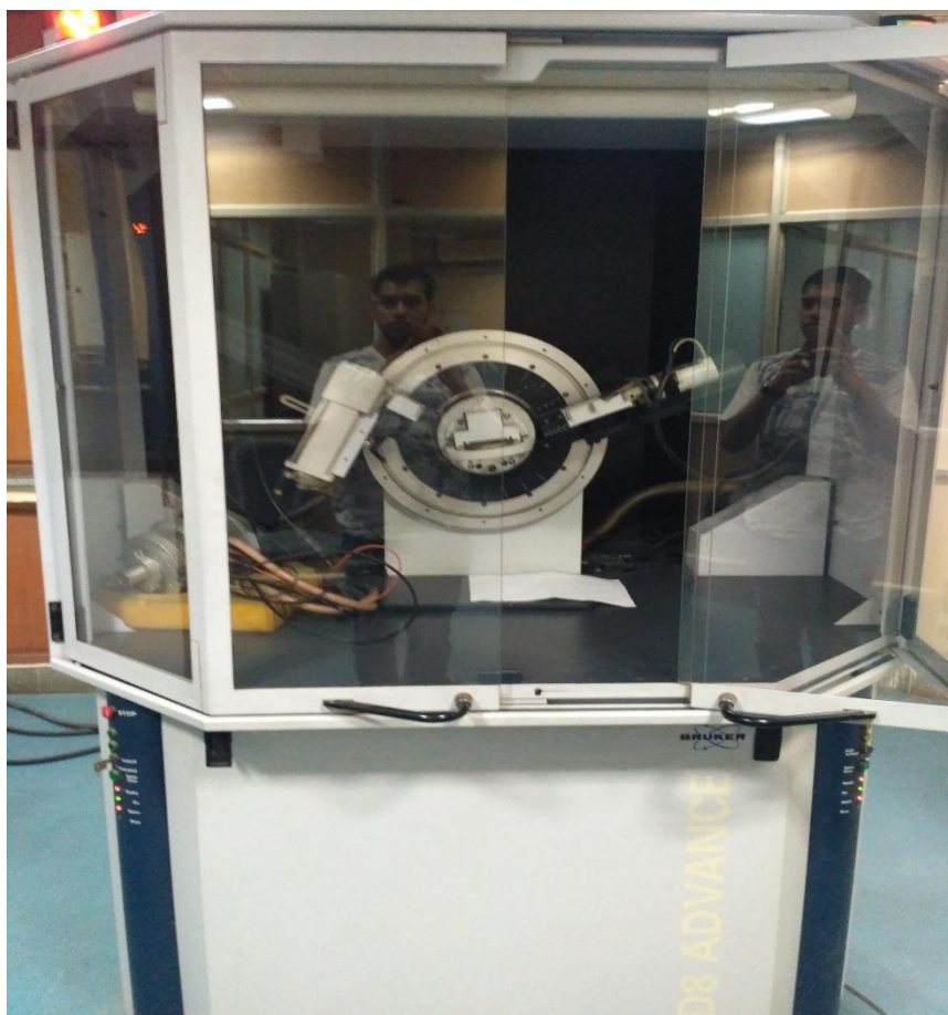
Fig. 3.12 X-ray Powder Diffractometer- Model: “Bruker D8 Advance” in Advanced Instrumentation Lab, Applied Physics Deptt., D.T.U.
