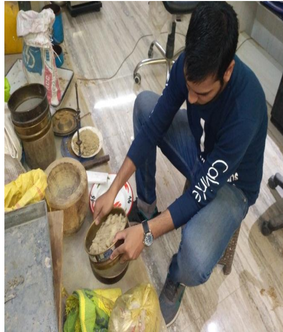
Fig. 3.8 Sieving the soil through I.S. 2 mm sieve
