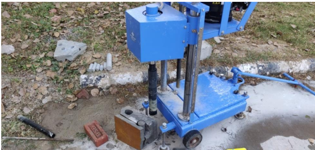
Fig 3.4- Extraction of rock cores from blocks with help of rock core cutting machine (concrete lab, DTU)
