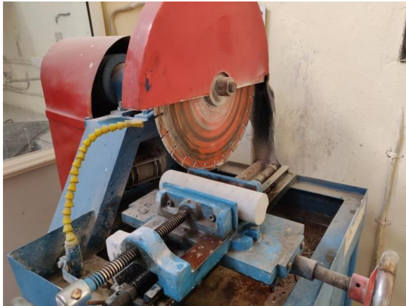
Fig 3.7- Sample preparation to suitable sizes for various tests, on rock cutting machine (Rock lab, DTU)
