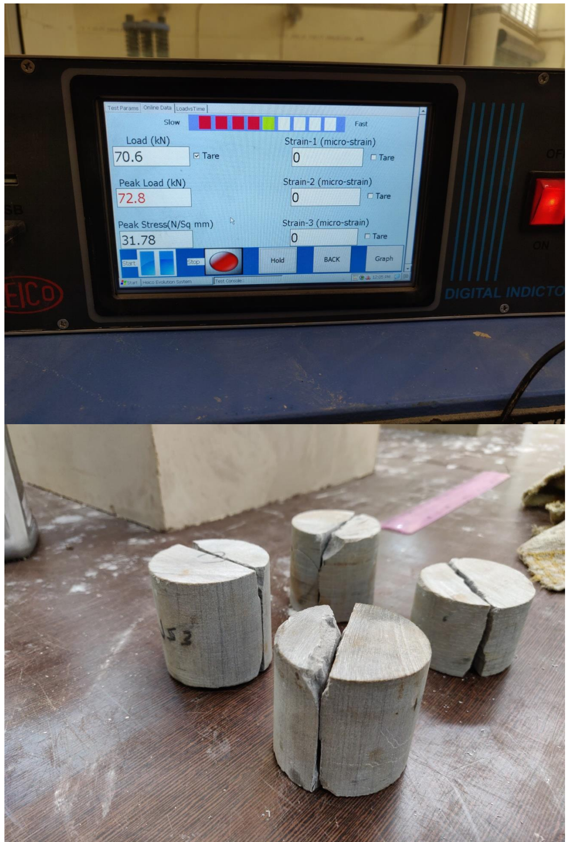
Fig 4.9- Value of peak load and samples after failure (Rock lab, DTU)
