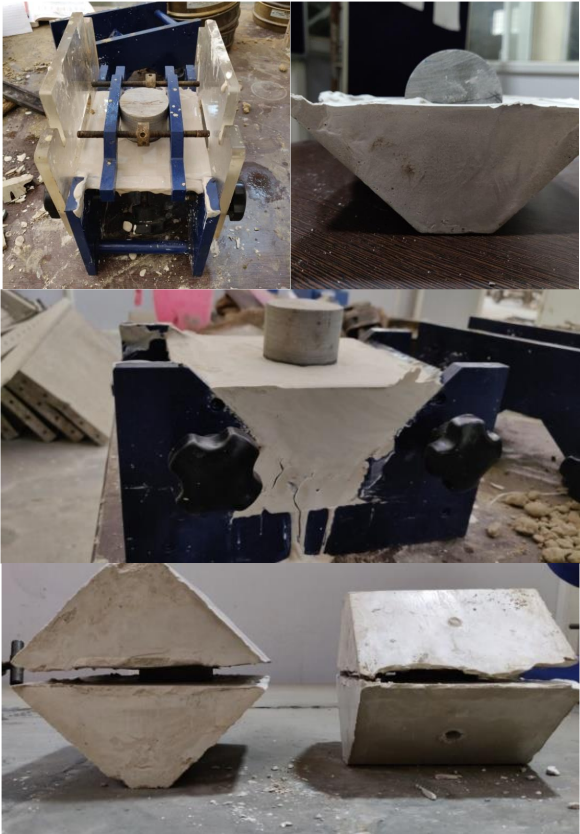
Fig 4.13 -preparation of samples for field shear test for intact rock core specimen shearing along the bedding planes (Rock lab, DTU)
