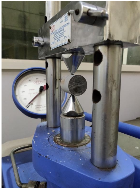
Fig 3.10 -Arrangement of rock core sample for testing for point load index (Rock lab, DTU)
