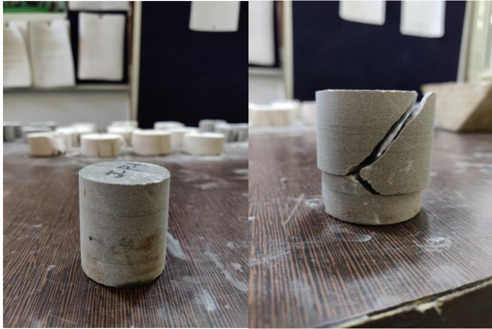
Fig 3.11 -Rock samples before and after testing for point load index (Rock lab, DTU)
