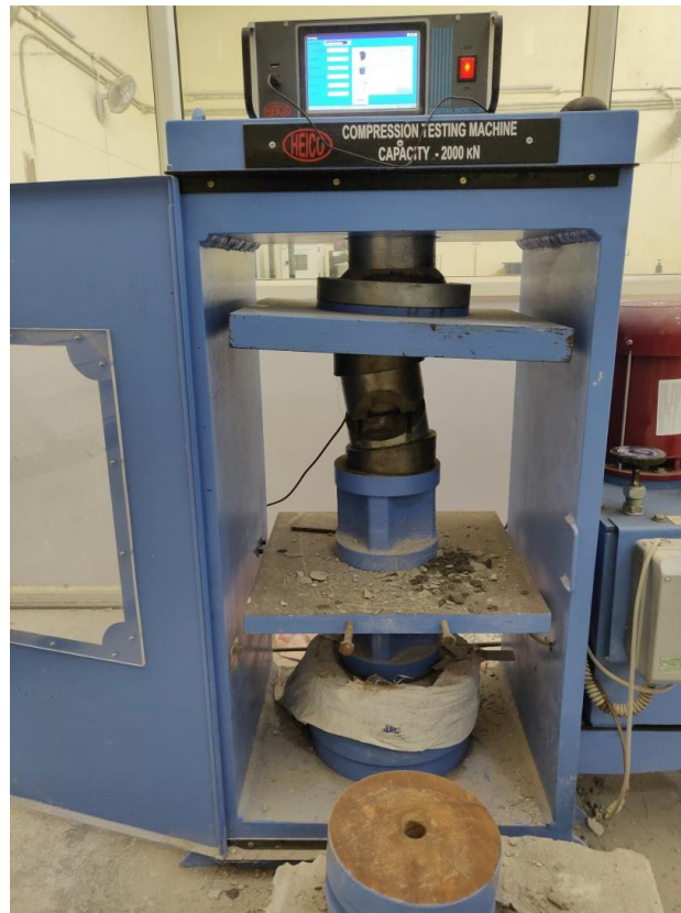
Fig 4.7- Application of normal load by CTM (Rock lab, DTU)
