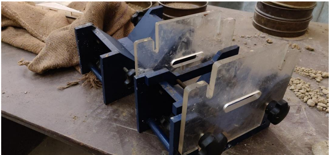
Fig 4.12 -Sampler used for preparation of samples for field shear test (Rock lab, DTU)
