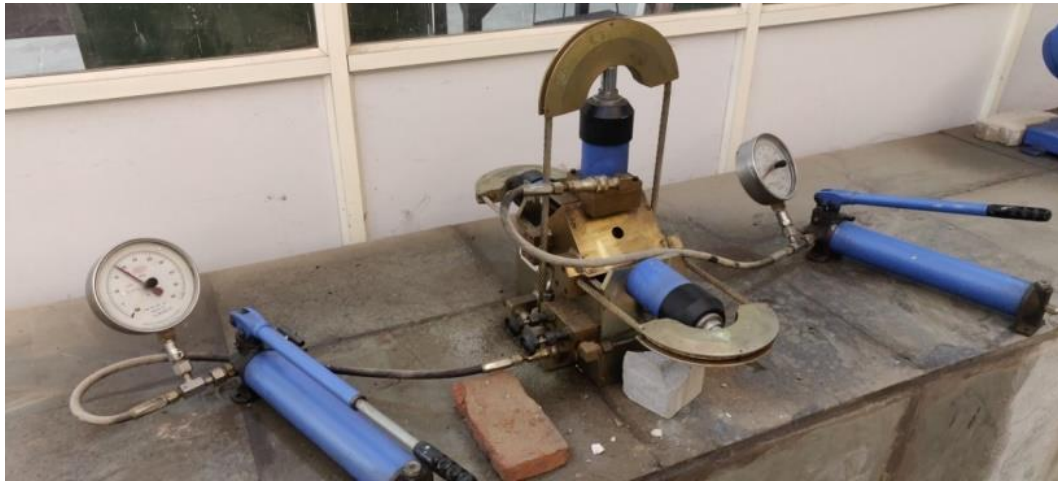
Fig 4.14- Testing the sample in field shear apparatus(Rock lab, DTU)
