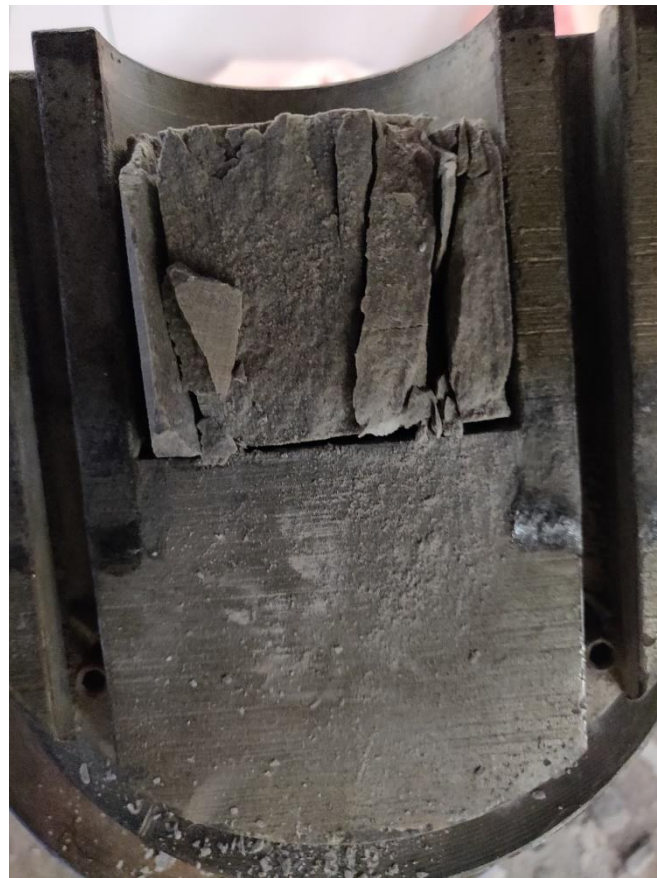
Fig 4.10 -Sample after failure when loaded at bedding planes being perpendicular to the direction of shear component of load (Rock lab, DTU)
