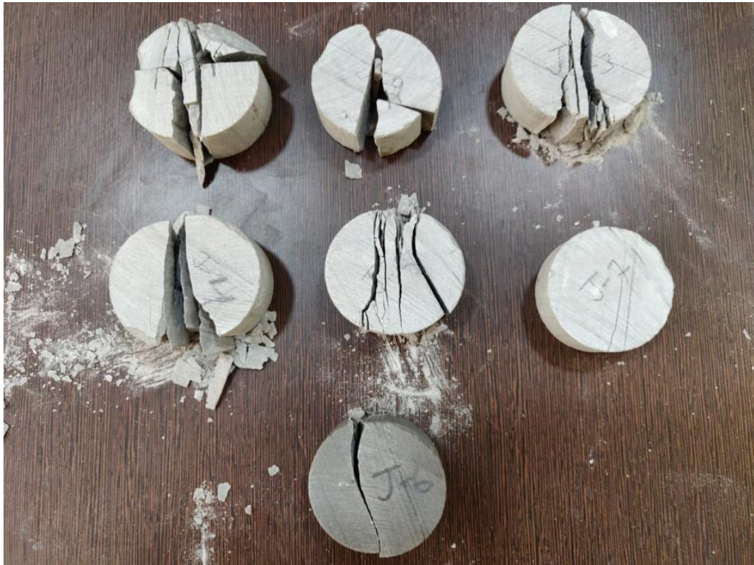
Fig 4.2- Different type of failure mode different angle of inclination( \theta=0^{\circ} - 90^{\circ} )
