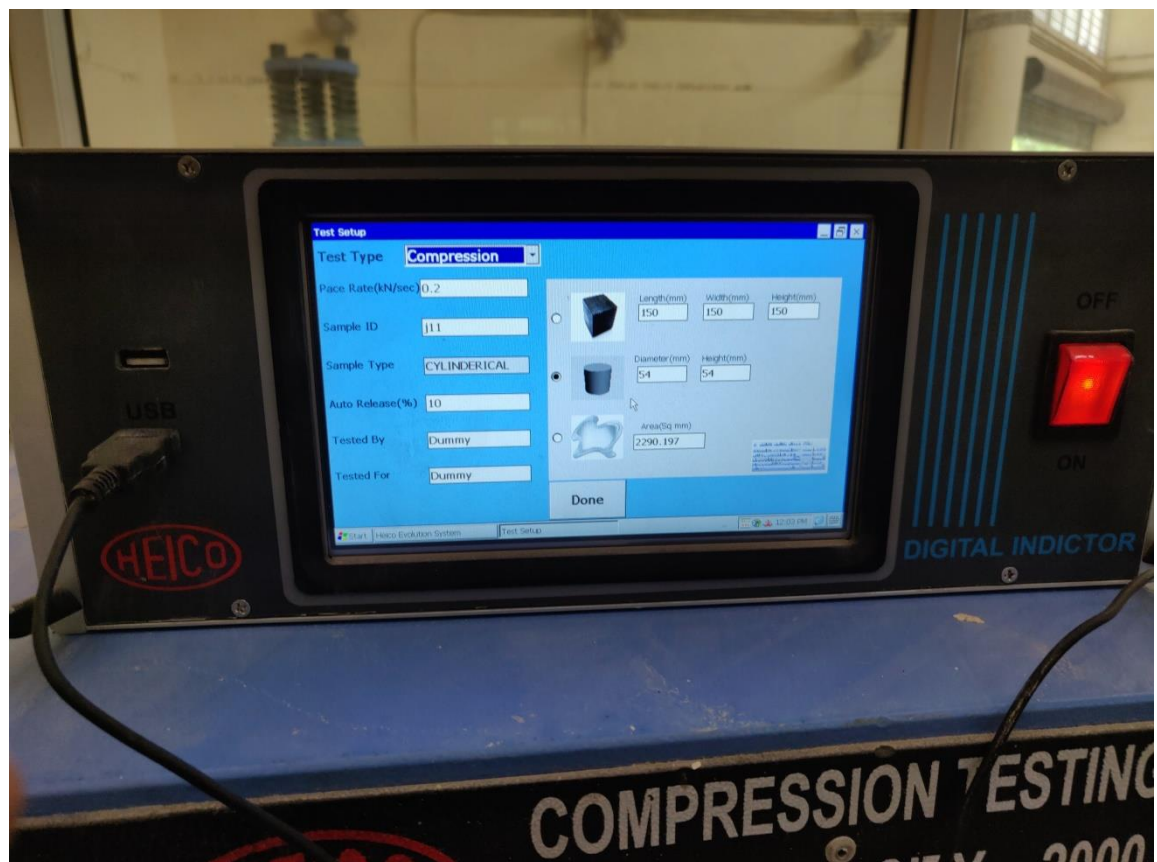
Fig 4.8-Arrangement for test, Data logger (Rock lab, DTU)
