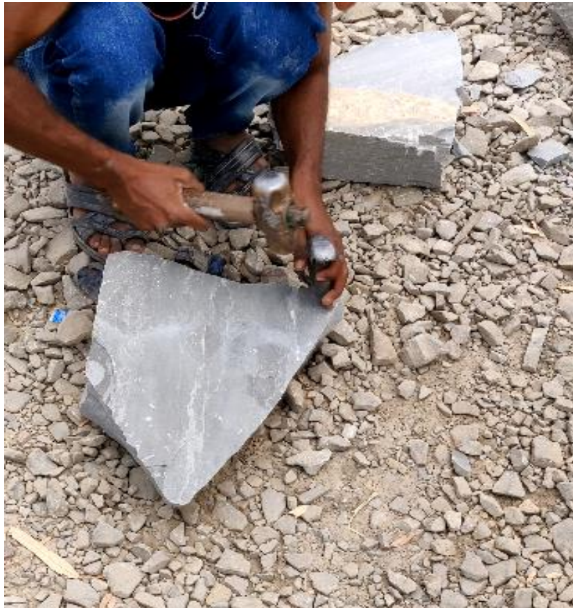
Fig 3.1- Dressing of stone with chisel and hammer (Dabi mines, Kota, Rajasthan)
