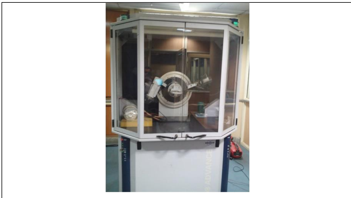
Fig. 3.17 X-Ray diffraction (Model: BRUKER D8 ADVANCED)
