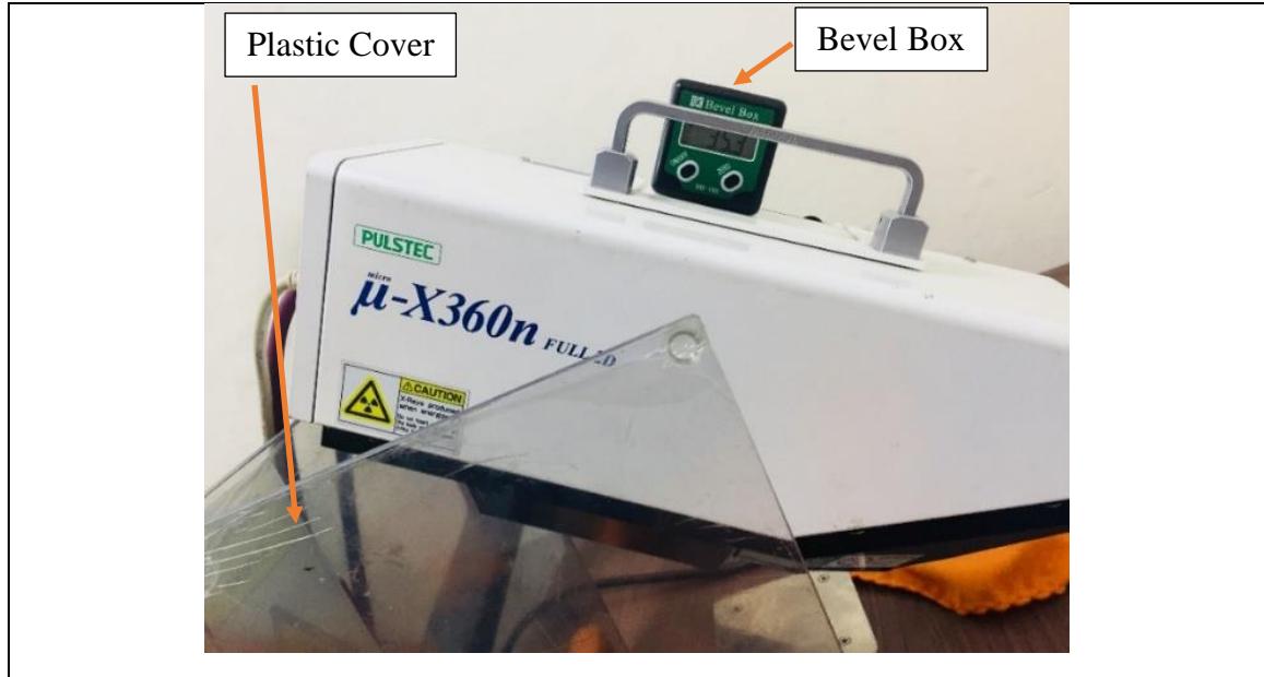
Fig. 3.18 Pulstec \mu -X360n Full 2D High-Resolution X-ray Diffraction (HR-XRD) machine
