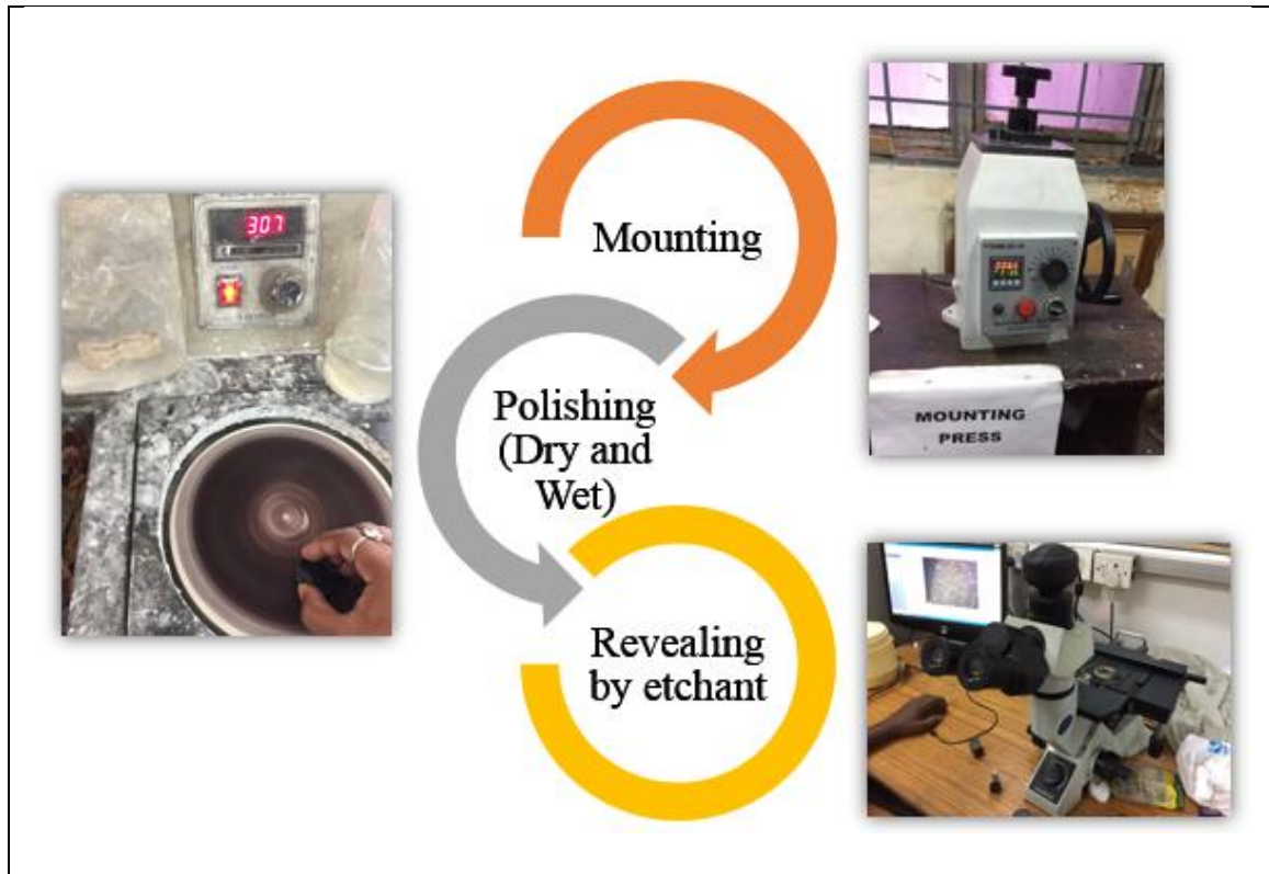
Fig. 3.8 Steps of sample preparation for microstructure characterization
