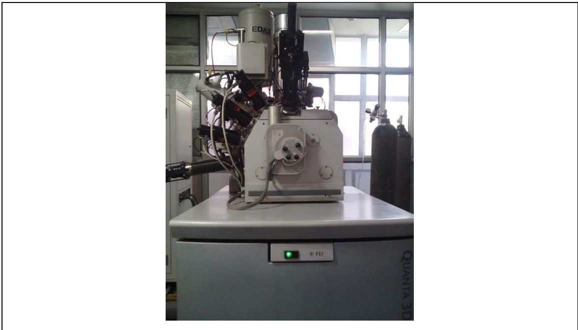
Fig. 3.16 Field Emission Gun Scanning Electron Microscope (FEG-SEM) (Model: FEI QUANTA 3D FEG)
