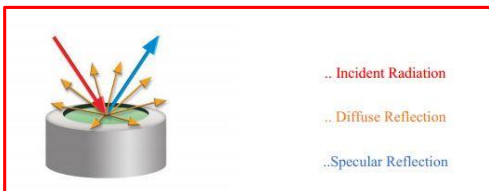
Figure 2.9. Incident and reflected beam through the sample under investigation
