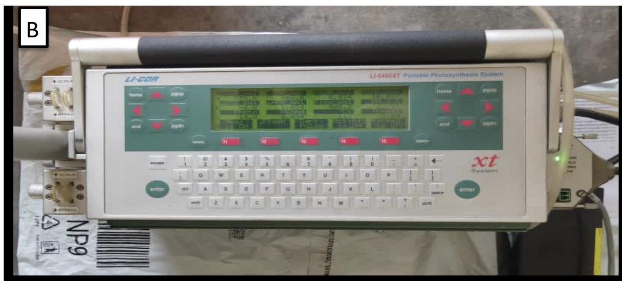
Figure 4.1- (A) Measurement of Physiological Parameters on IRGA (B) portable photosynthesis system Li-6400XT IRGA
