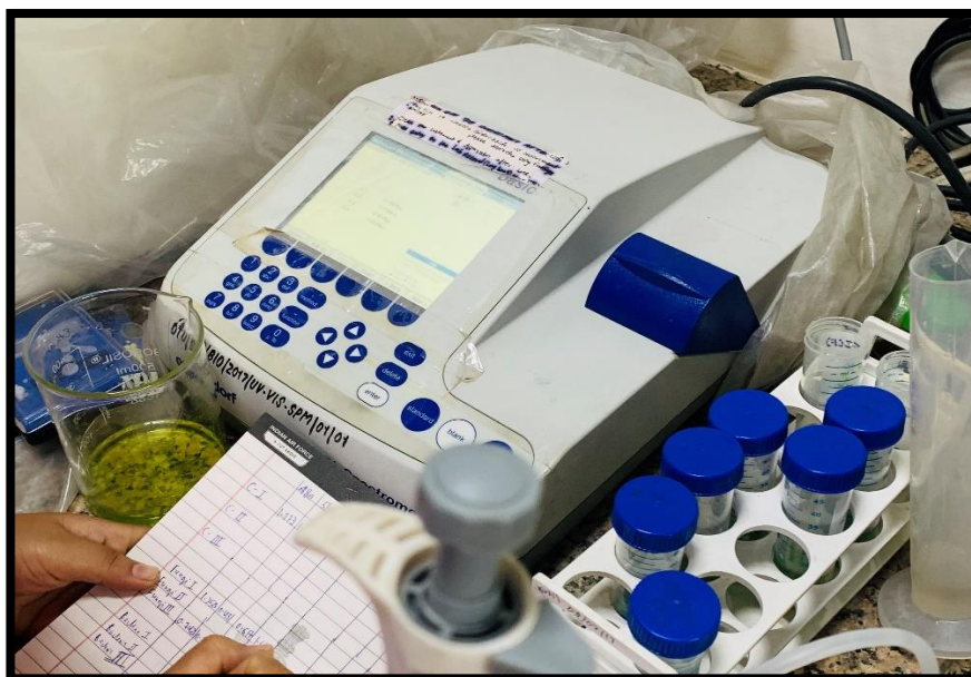
FIGURE 4.2- Measurement of Absorbance of Leaf Extracts on UV spectrophotometer for Estimation of Chlorophyll and Carotenoid content
