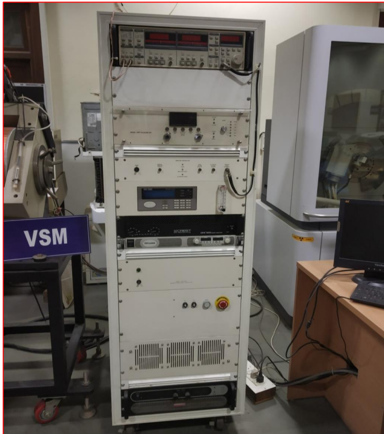
Figure 2.8. Vibrating Sample Magnetometer (VSM) setup.
