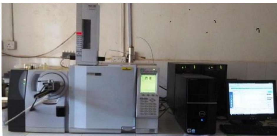
Plate 3.12 GC-MS test setup
