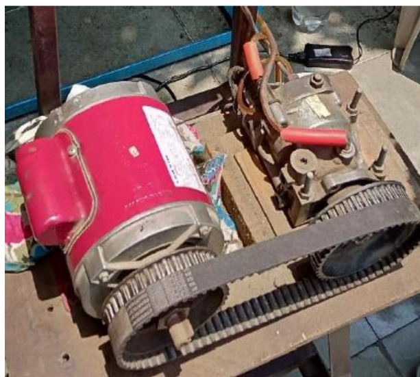
Plate 3.15 Fuel pump connected to the motor
