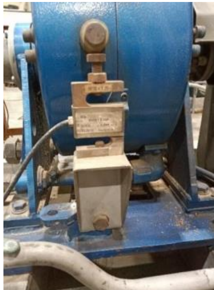
Plate 3.21 Load cell placed on the dynamometer
