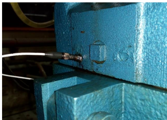
Plate 3.25 Pressure sensor installed on the engine head
