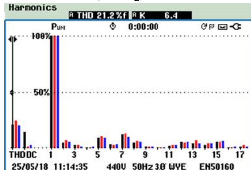
Fig. 6.6(c): Current THD at ESS (off-grid) side of ADSIG-Mode 3
