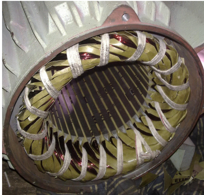
Fig. 3.15 Empty Stator Induction Motor Wounded as ADSIG
