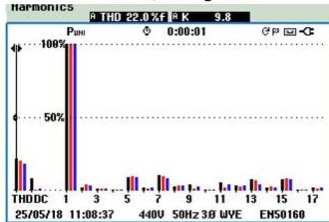
Fig. 6.5(c): Current THD at ESS (off-grid) side of ADSIG-Mode 2
