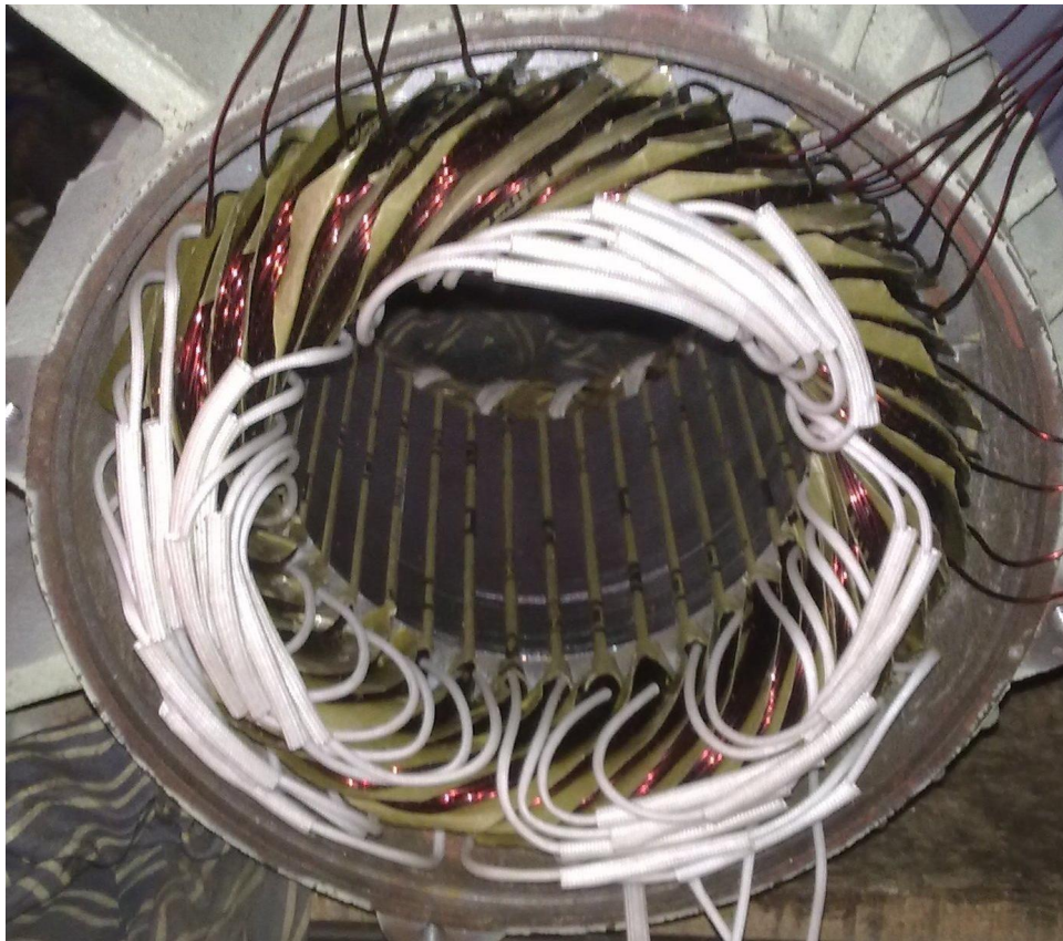
Fig. 3.14: Rewinding of Empty Stator Induction Motor
