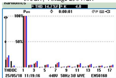
Fig. 6.7(c): Current THD at ESS (off-grid) side of ADSIG-Mode 4
