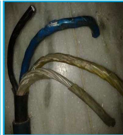
Issues: cracking of R,Y & B ph XLPE insulation & moisture ingress in conventional design
