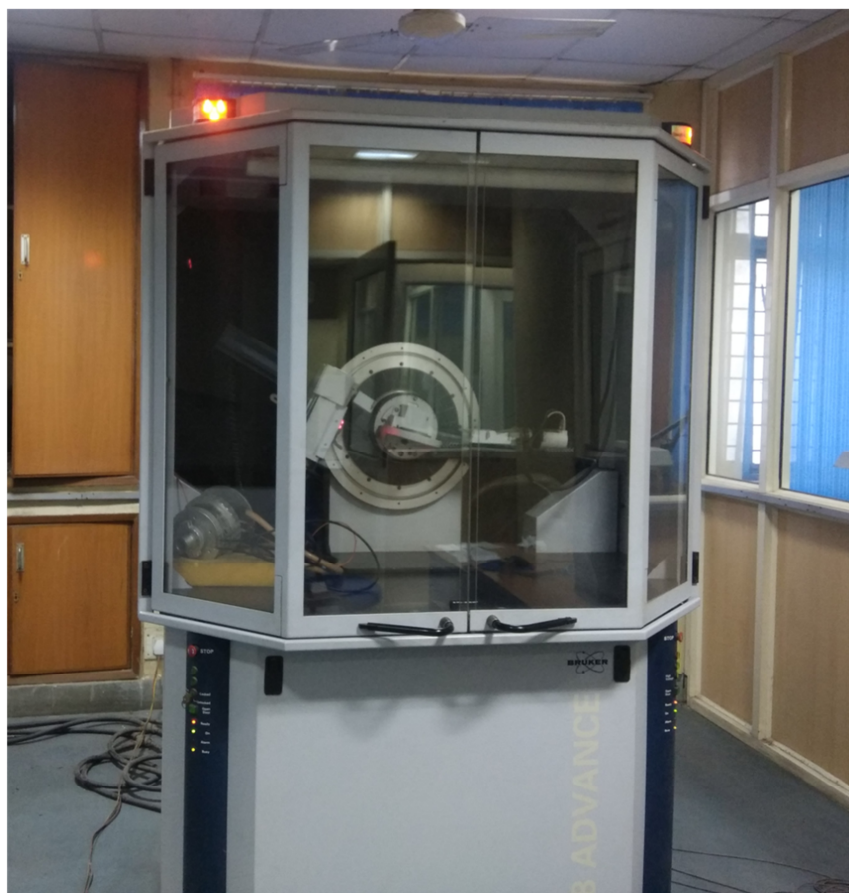
Figure 2.5: Set-up of X-ray diffraction (XRD)
