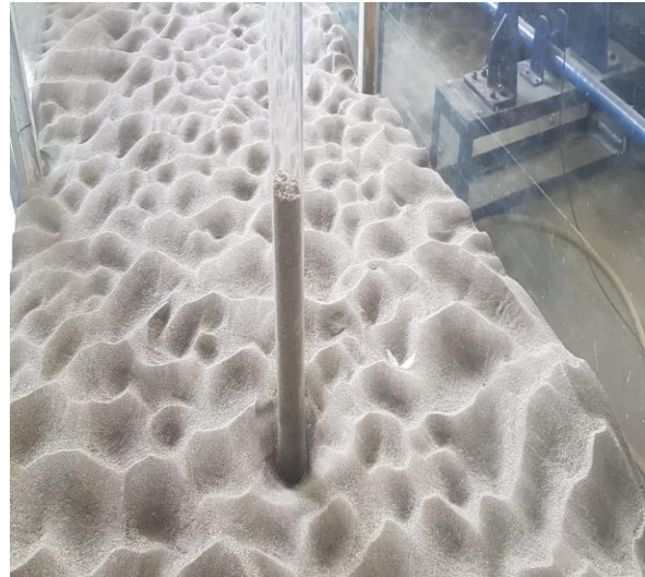
Figure 15 Types of circular collar and surface profile after experiment
