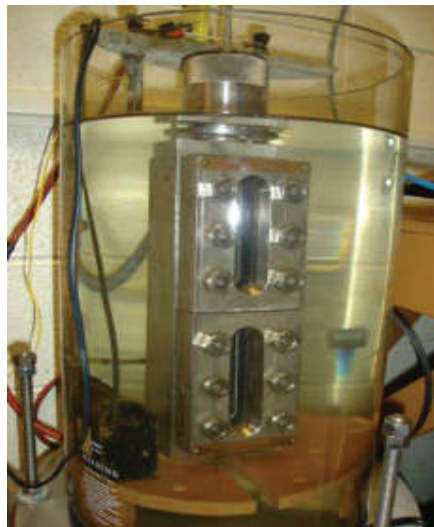
Plate 6: Thermal bath with high pressure test chamber [16]
