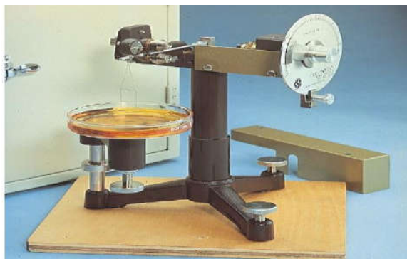
Figure 2: Du Nuoy Ring Tensiometer [6]
