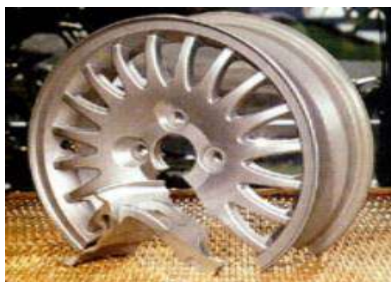
Figure 1.5: Dissimilar Aluminum Alloy Wheel (Courtesy: Wheel assemblies using two aluminum alloys have been made by Hydro Aluminum in Norway)
