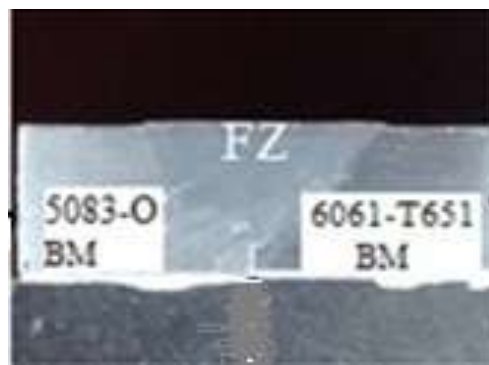
Figure 7.3: Sample after Polishing and Etching
