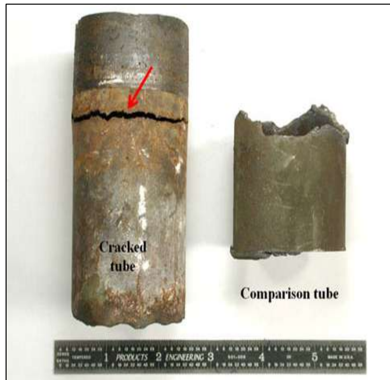
Figure 1.13: Tube Breaking Under Stress Corrosion Cracking [3]
