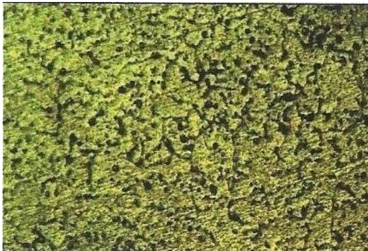
Figure 7.8: Microstructure of HAZ at 6061-T651 side at 200X
