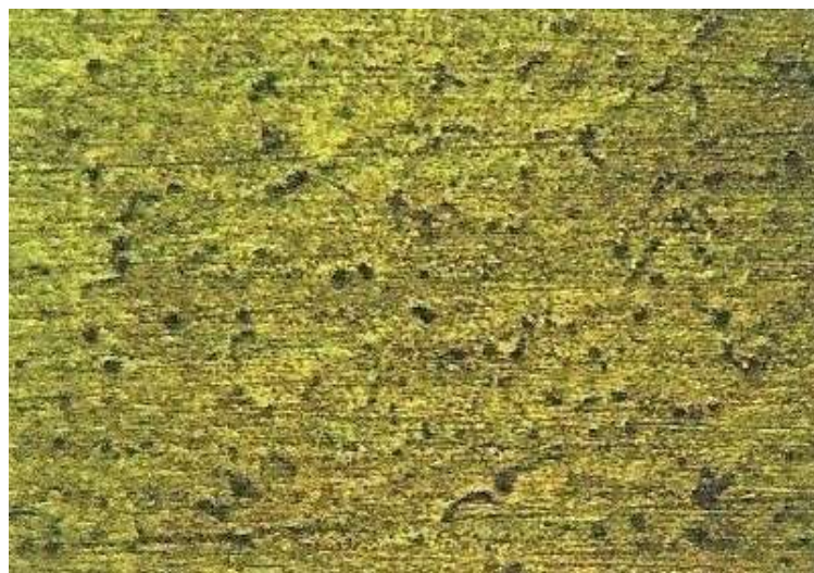
Figure 7.7: Microstructure of HAZ at 5083-O side at 200X
