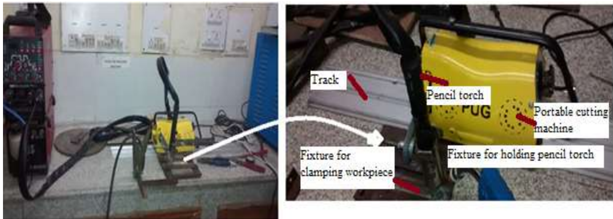
Figure 3.3: Torch Mounted on Trolley Moving on Dedicated Track
