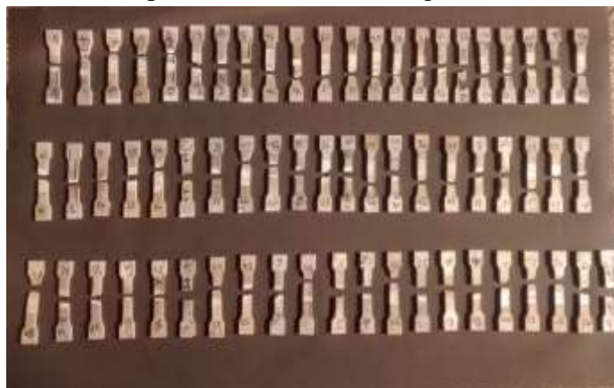
Figure 5.9: Tensile Tested Specimens Showing Location of Fracture
