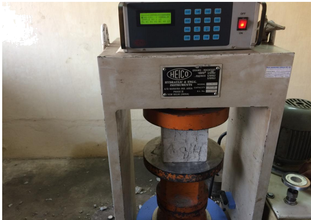
Plate 3.5 Test Set up for Compression Test
