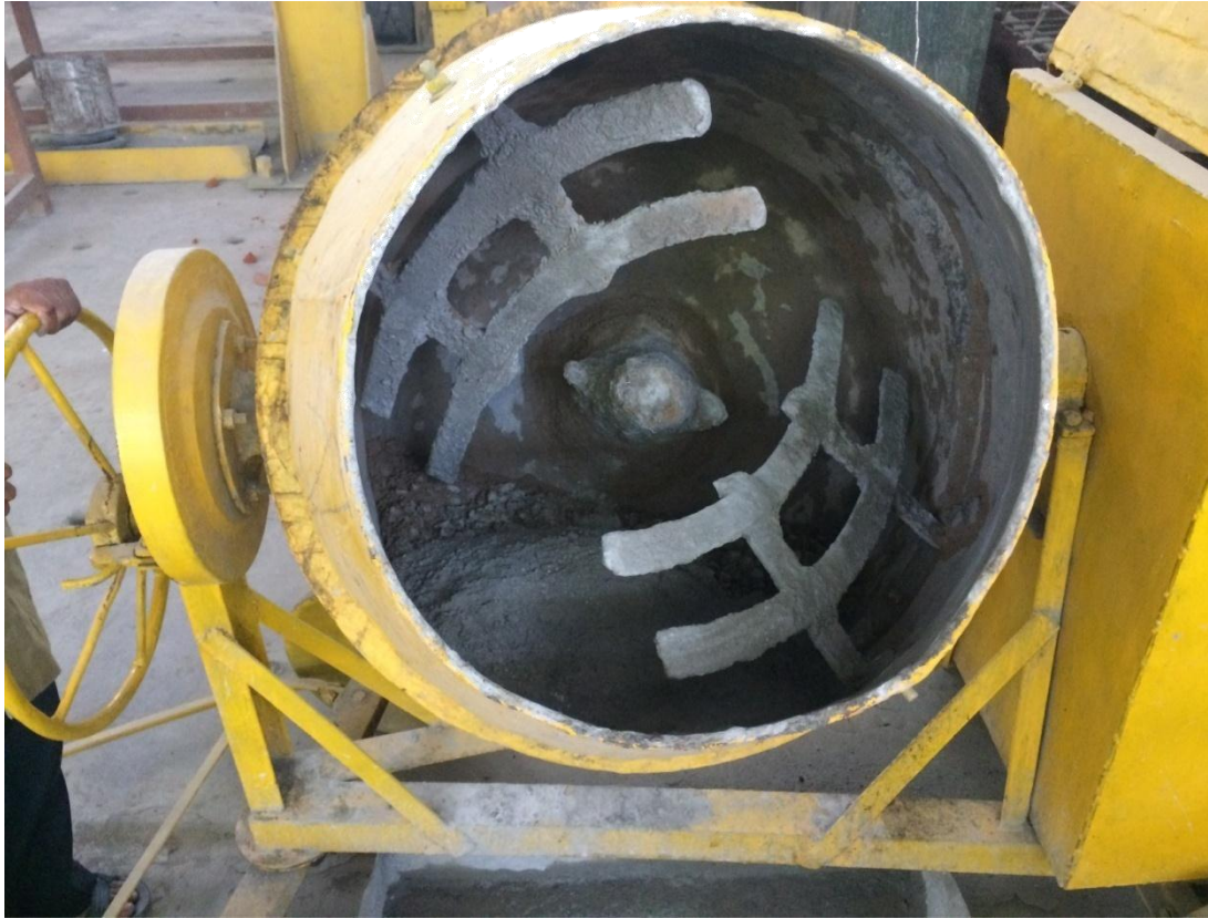
Plate .3.2: Mixing of materials in the mixer
