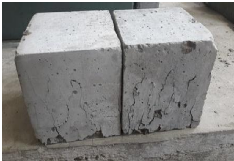
Plate 3.6 Cracks developed after testing in cubes
